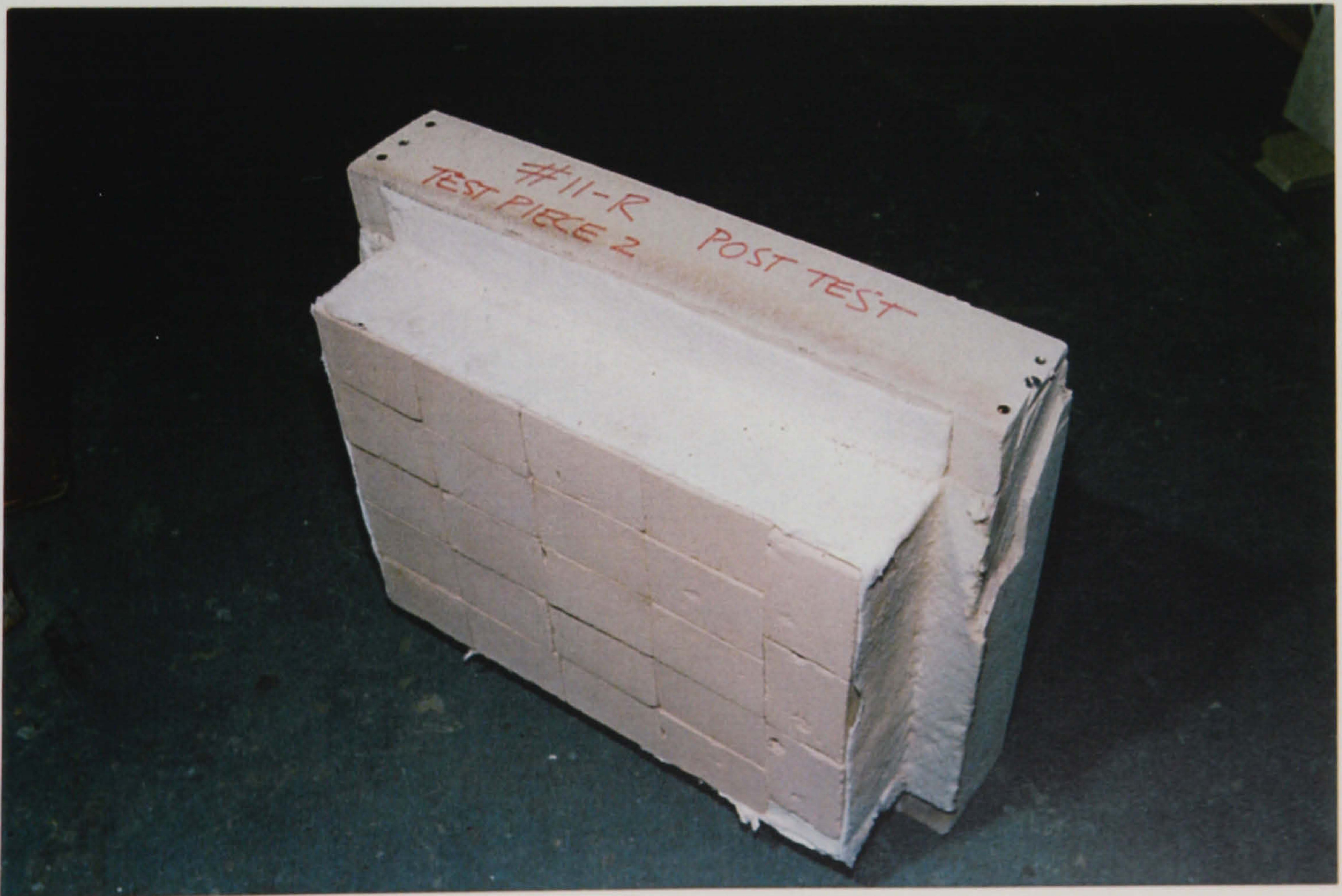
Figure A.5.10 Post test condition of Insuline #11-R samples
