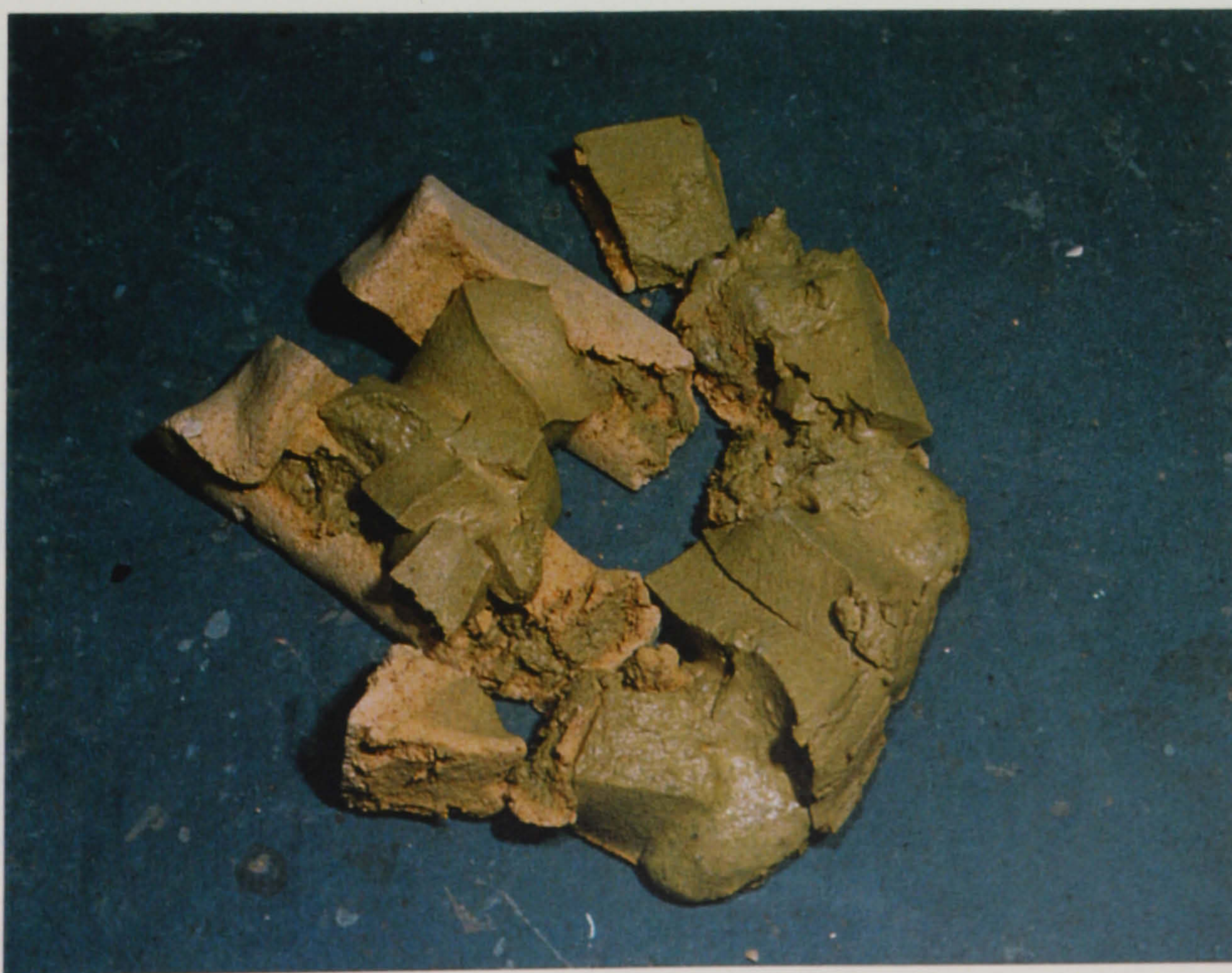
Figure A.4.10 - Condition of #11-R samples after heating to 1300°C
