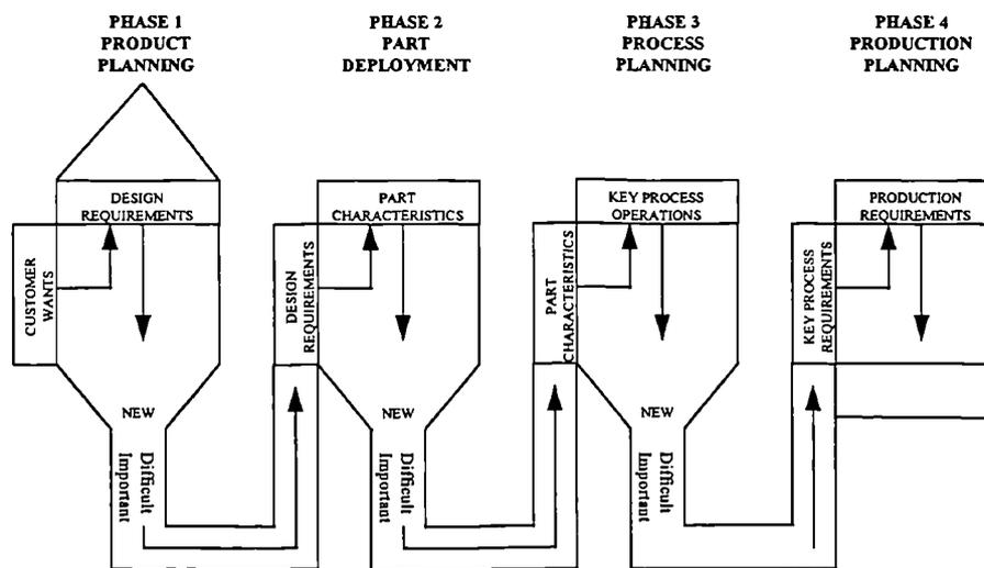
Figure 5.10: the four phases of QFD for manufacturing industries
