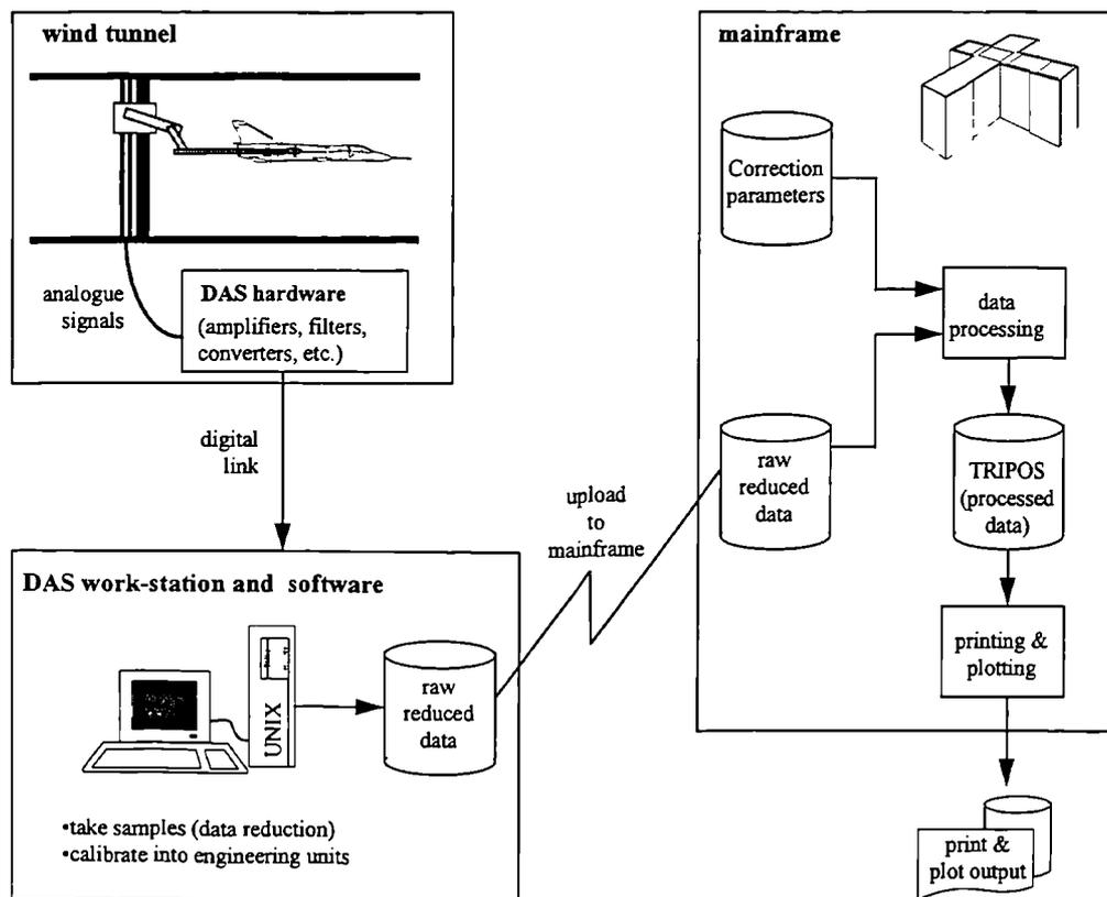
Figure A.3: LSWT - current computing environment and data-flow
