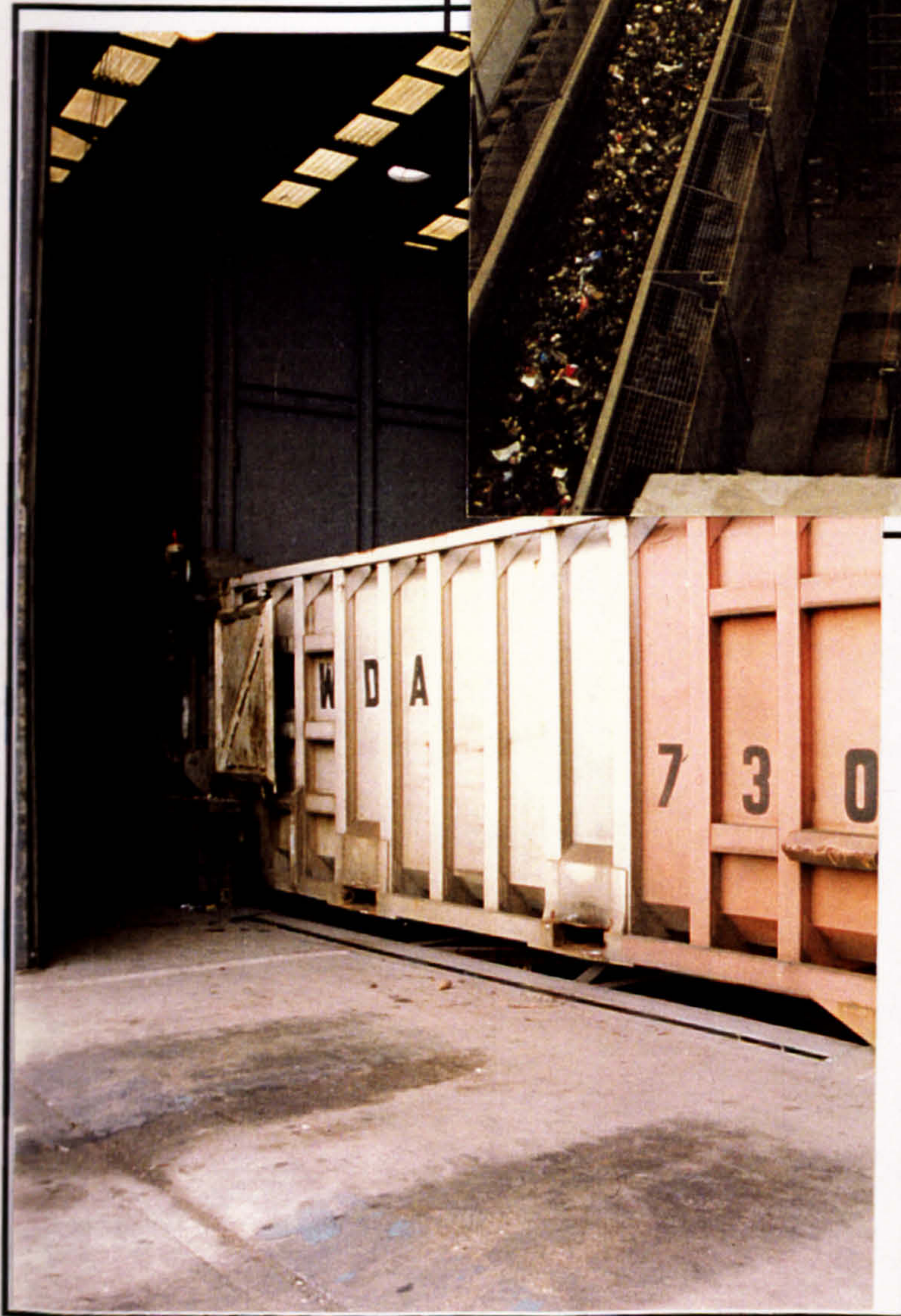
Plate 2-8: An example of a 20 tonne container used in the transportation of the bulky wastes or the contraries
