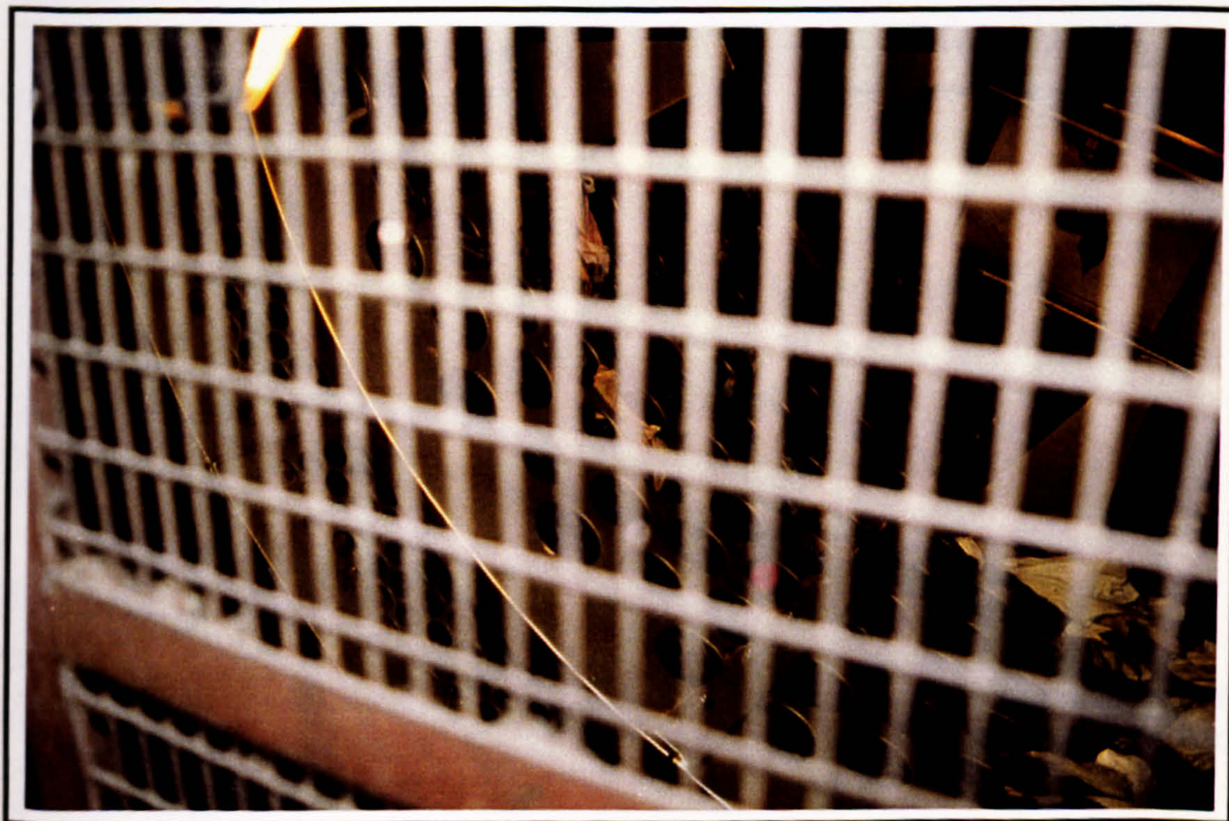
Plate 2-6: The wastes is separated into fine and coarse contraries by the two different size of sieve plate at the end of the drum
