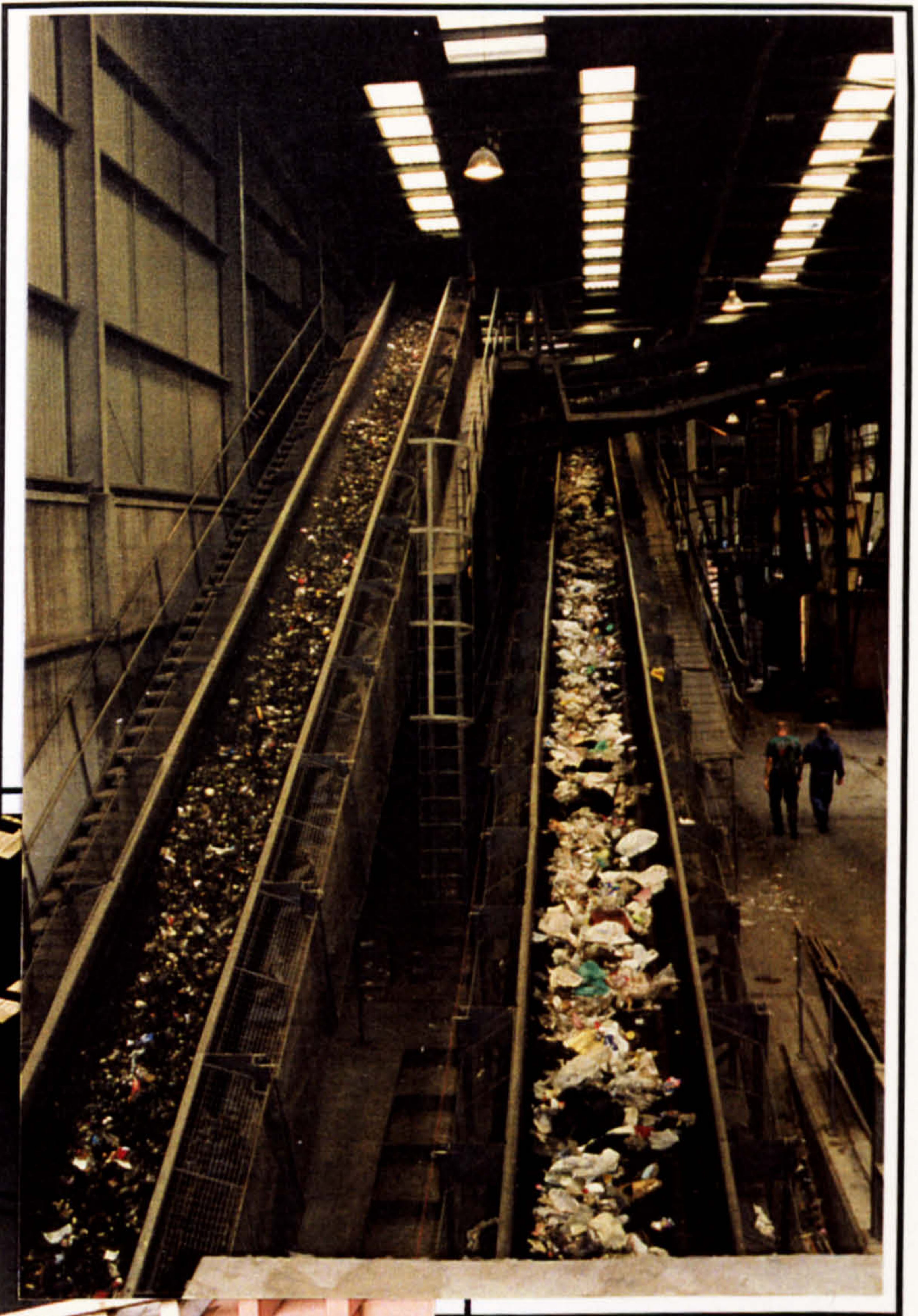
Plate 2-7: The fine and coarse contraries conveyor belt from the drum up to the metal separating unit at the top.
