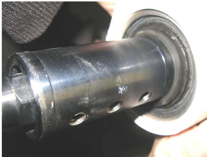
**Figure 8: Photograph of Turbine 1 connection point. The stub is designed to be inserted into a mounting pole**
