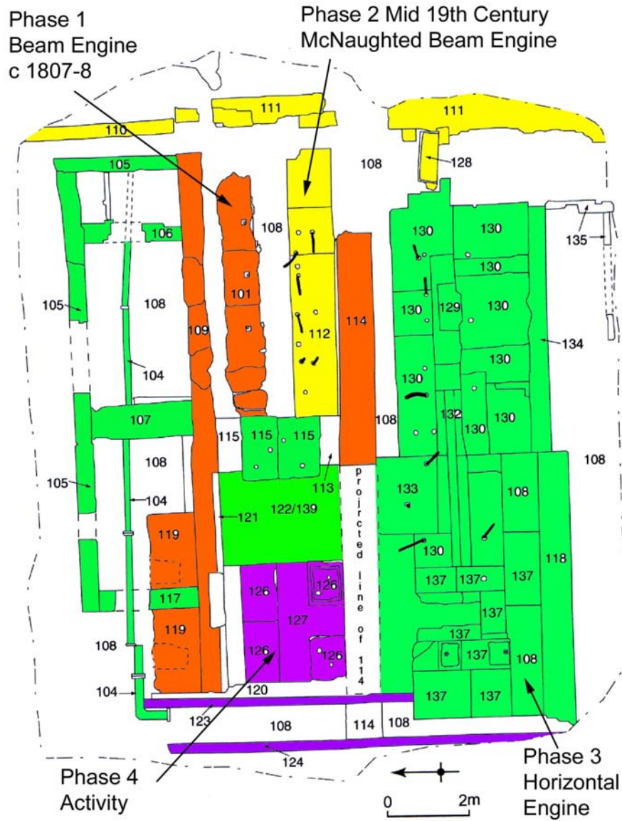
Fig. 121. Portwood Mill: Phased plan of the engine house.
