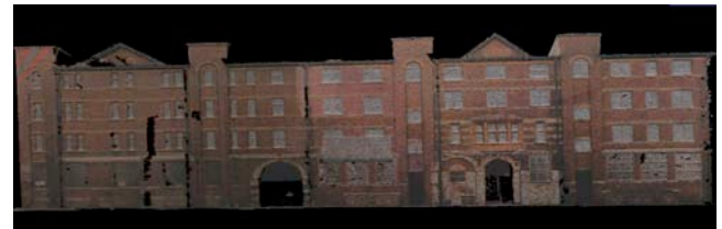
Figure 2: Virtual Reality (VR) model produced from raw scan data
