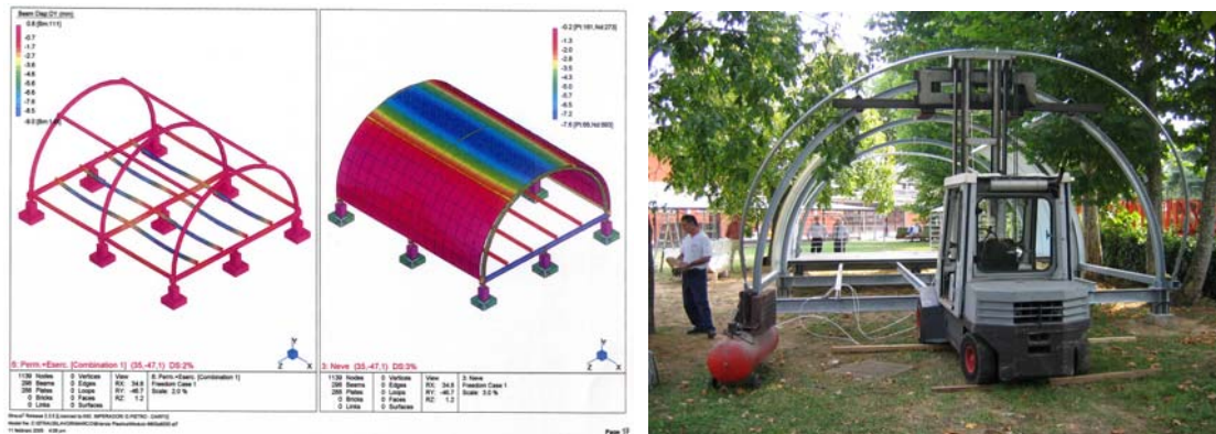
Figure 10,11 The structural system has been calculated with Straus automatic finite elements program both for stress and strains. A test programme has been carried out to verify the theoretical calculations.
