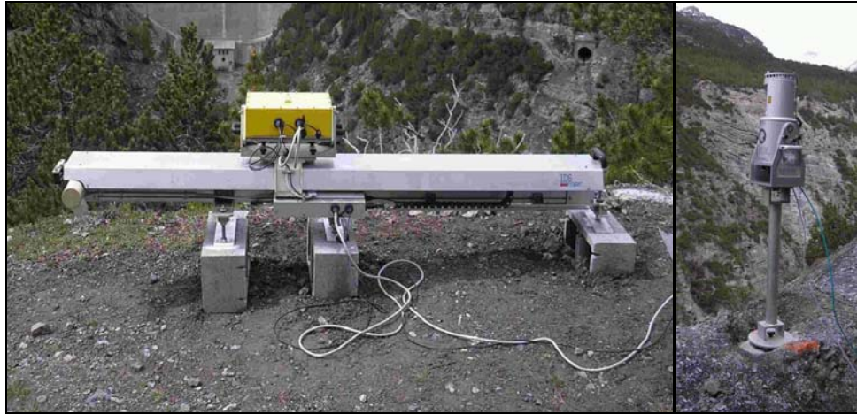
Figure 2: On the left a GB-In SAR system IBIS-L by IDS (Pisa, Italy); on the right a long-range terrestrial laser scanner Riegl LMS-Z429i mounted over a steel pillar for precise repositioning.
