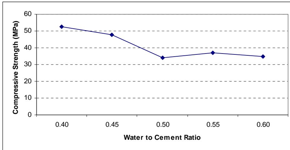
Figure 2. Compressive Strength of RAC at 28 days
