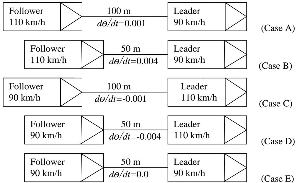
Figure 2. Illustration of positive, negative and zero angular velocities
