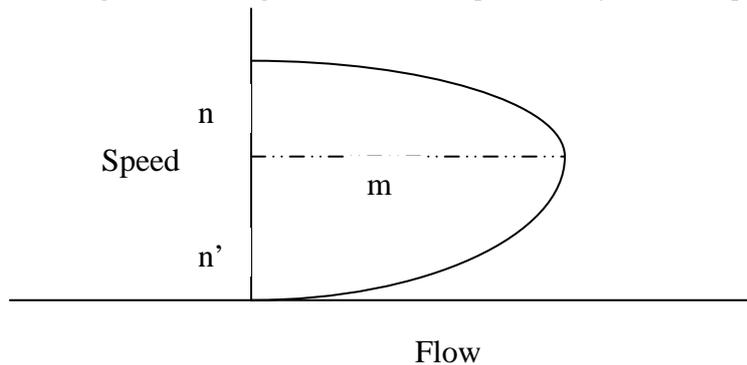
Figure 4 Speed-flow for the two-regime linear speed-density relationship
