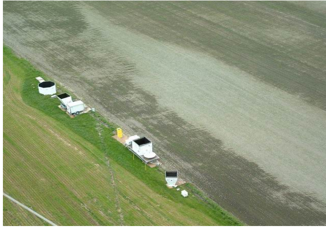
Figure 15. The three SODARs used for calibration. From upper left: Scintec SFAS (octagonal baffle), AV4000 (small square baffle), and Metek SODAR/RASS (large square baffle). The fourth SODAR, lowermost in the picture, was not used for calibration.
