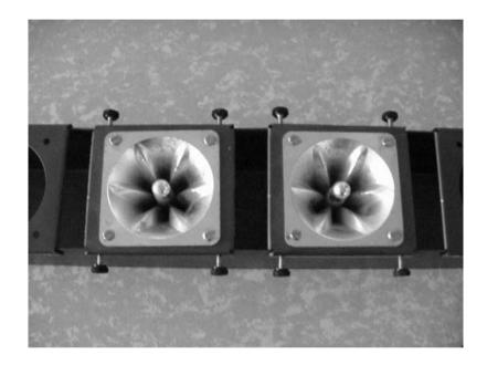
FIG. 8. Adjustable linear array configuration.
