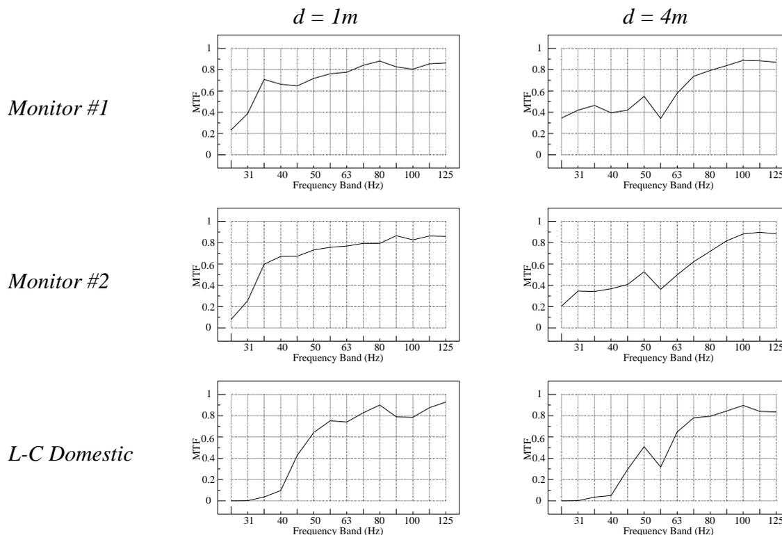
Figure 2 MTFs of 3 Loudspeakers in a Reasonably Well Damped Studio Recording Room at Different Distances  $d$  from the Loudspeakers
