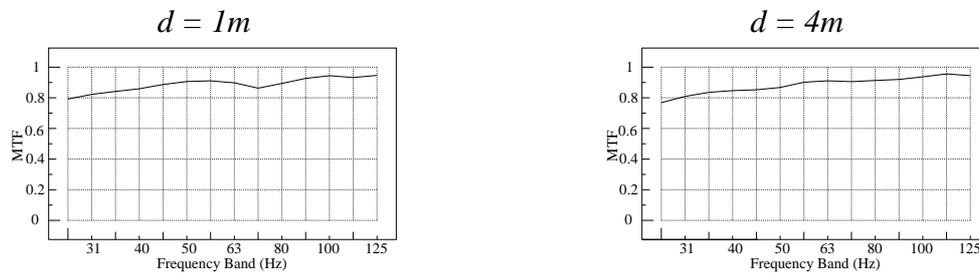
Figure 1 MTFs of a Wide Range Monitor System in a Very Highly Damped Studio Control Room at Different Distances  $d$  from the Loudspeaker
