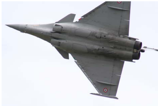
Figure 1 Leading-Edge Slats Deployed on Dassault Rafale Aircraft
