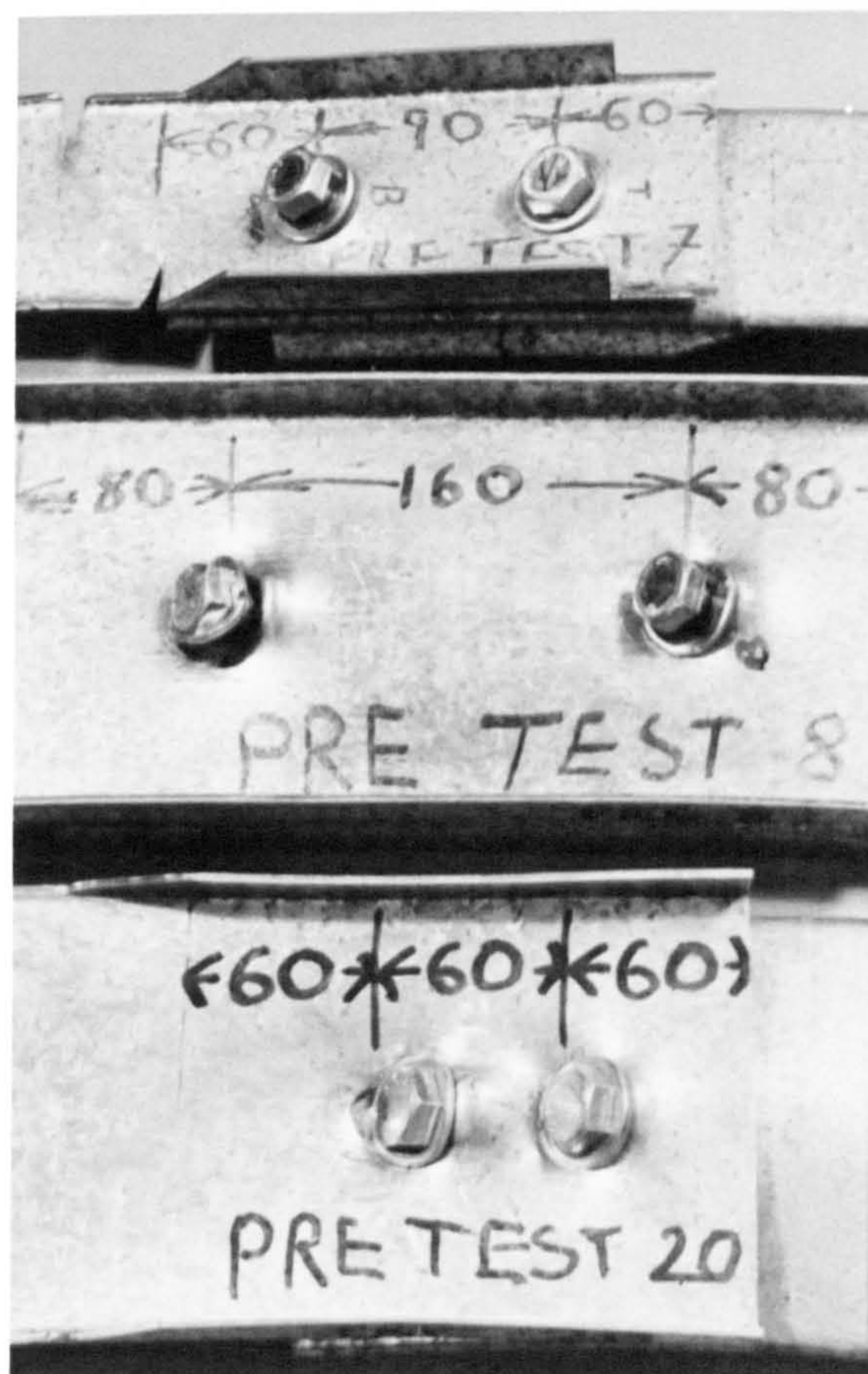
Fig. 3-7. Lap joints with two bolts in line of stress
