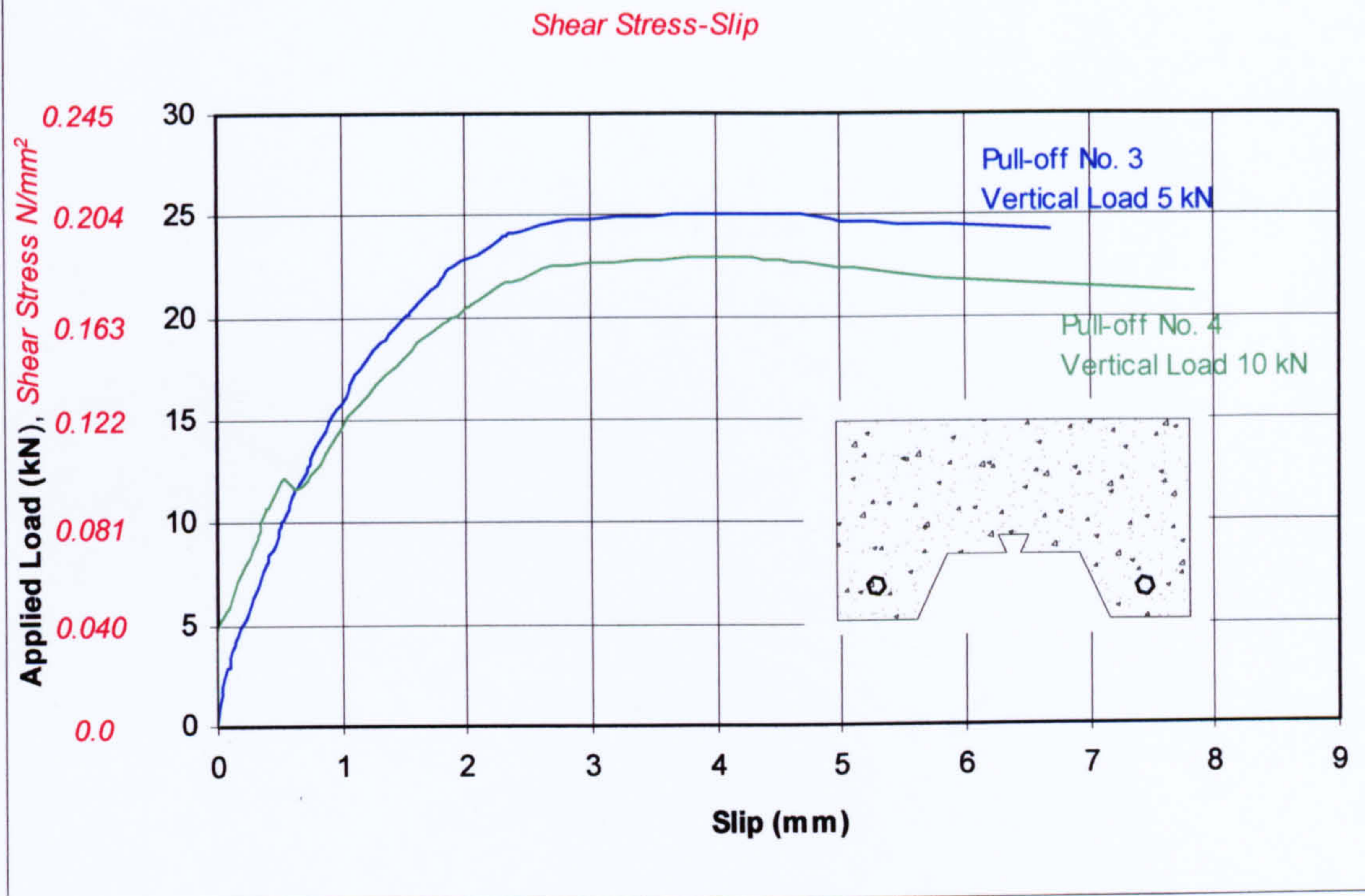
Figure 3.22 Comparison of Pull-out test No. 3&4 (Load-Slip)
