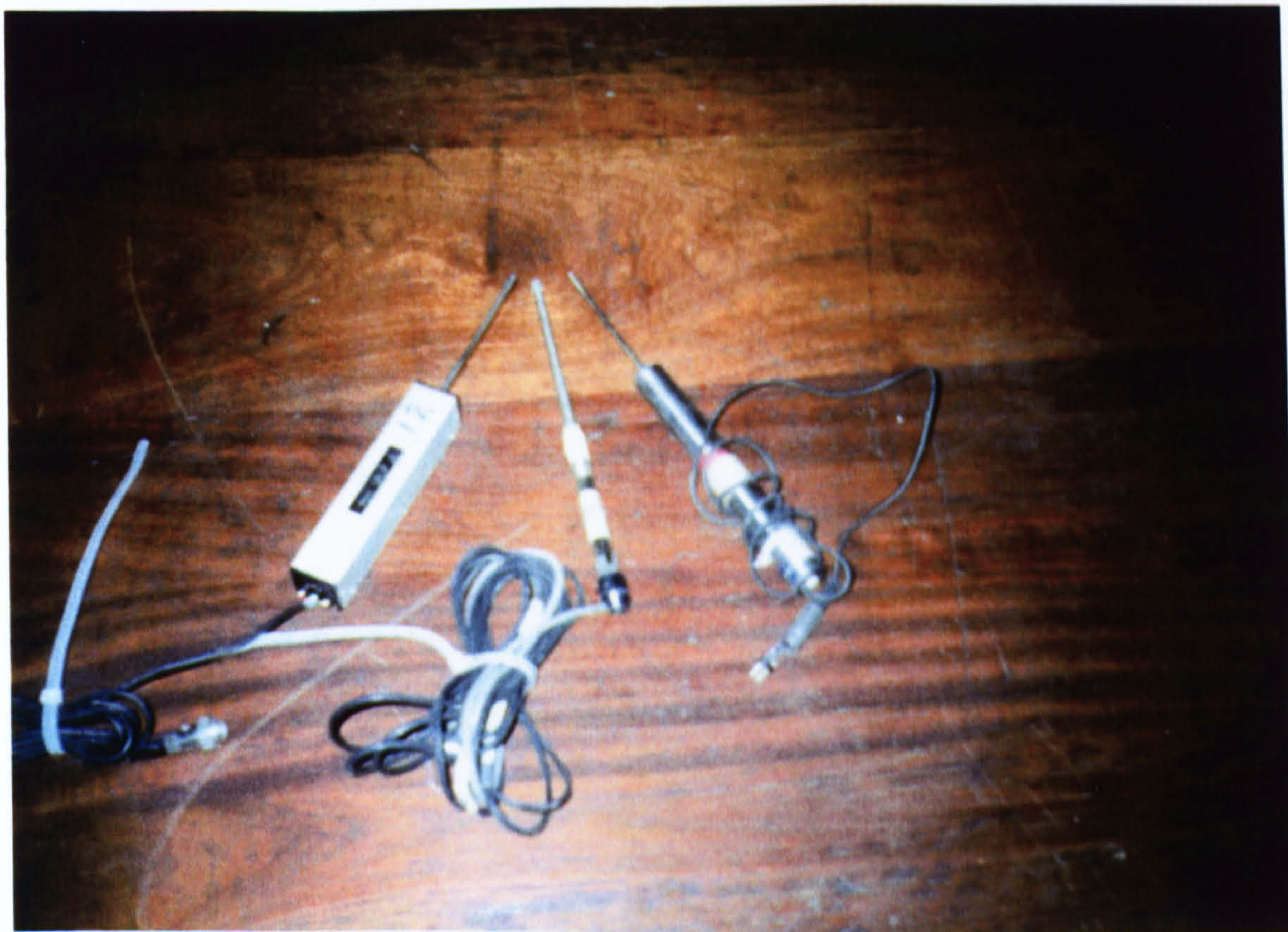
Plate 2. Deflection Gauges (LVDTs)
