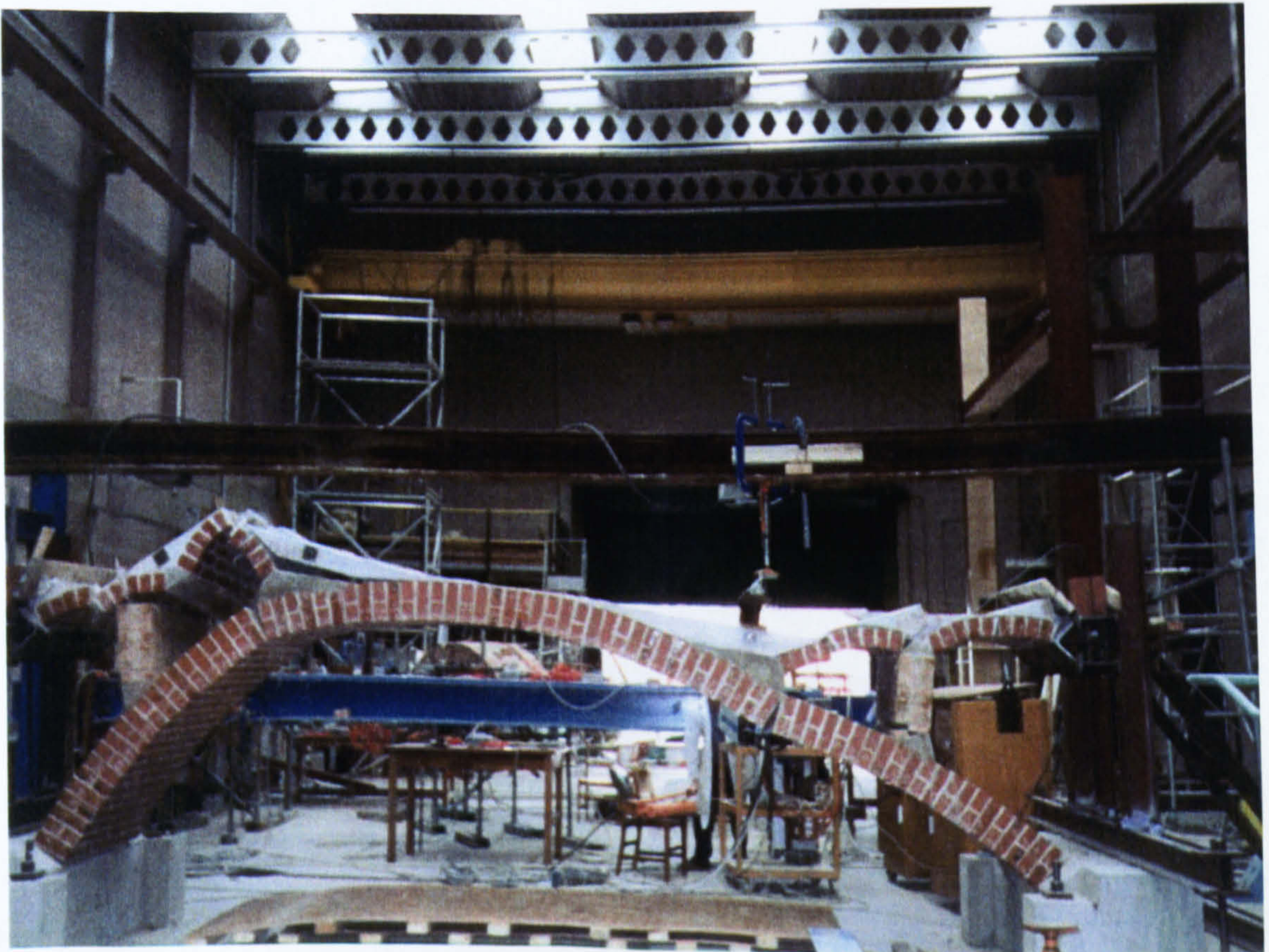
Plate 10. Failure Mechanism of The Model OSMA5
