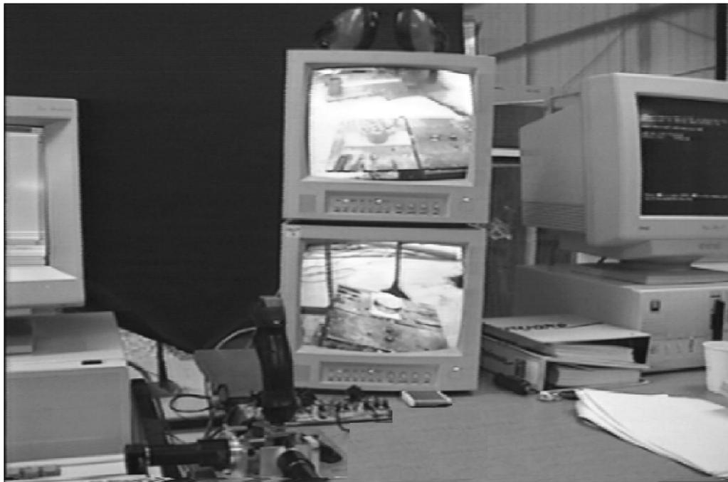
Figure 6.2: View of the operator workstation, showing the camera monitors and the haptic joystick
