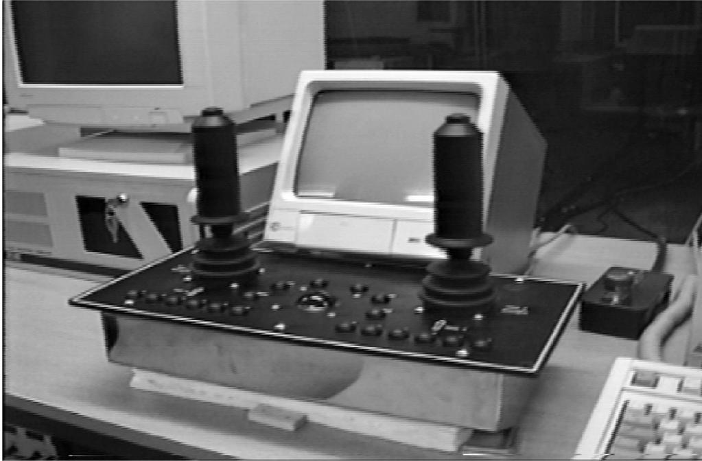
Figure 4.2: The UK Robotics Ltd Advanced Teleoperation Controller
