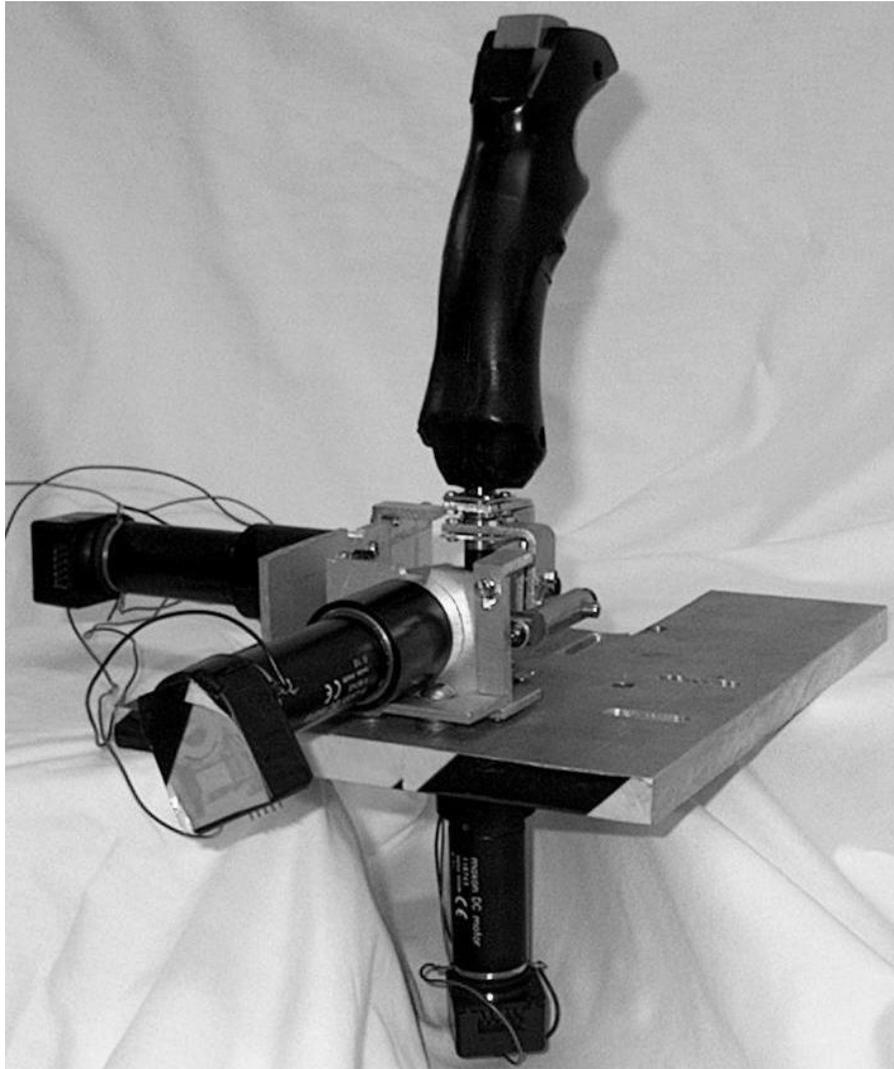
Figure 4.17: The complete three degrees of freedom haptic device
