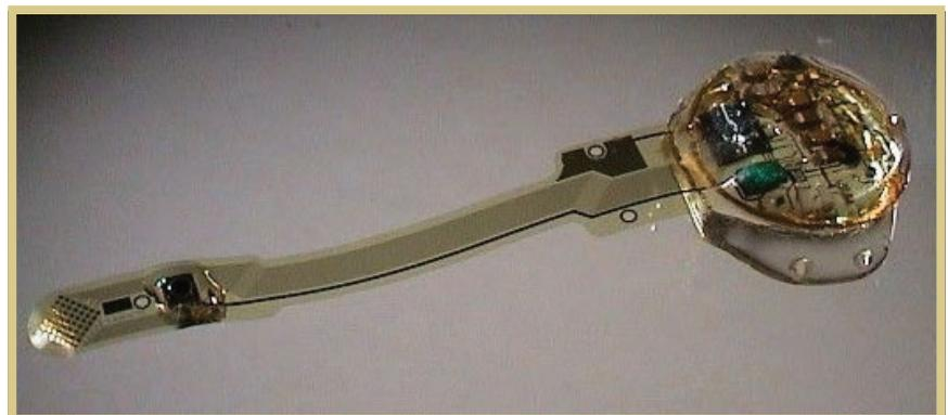
Figure 2. Retinal stimulator for the Healthy Aims retinal implant system. The electrode array is 4 × 5.5 mm, and the electronics is approximate 25 mm in diameter.
