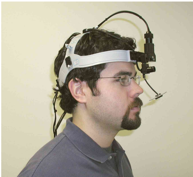
Figure 2. ASL H5 Head Mounted Eye Tracker
