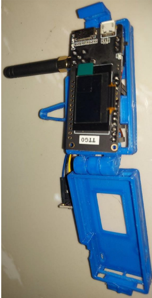
Fig. 3. 3-D printed enclosure housing the payload.
