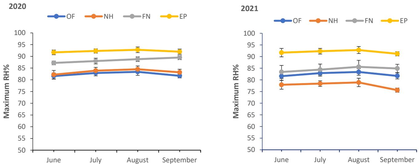
**Figure 6.** Average monthly maximum relative humidity percentage (RH%) during the experiment periods of 2020 and 2021 seasons, registered in the open field (OF), net house (NH), net house with fogging (NF, operating 6 S/36 S from 10 a.m. to 4 p.m.) and evaporative cooling under plastic house (EP). Standard error of the means was derived three biological replicates.
