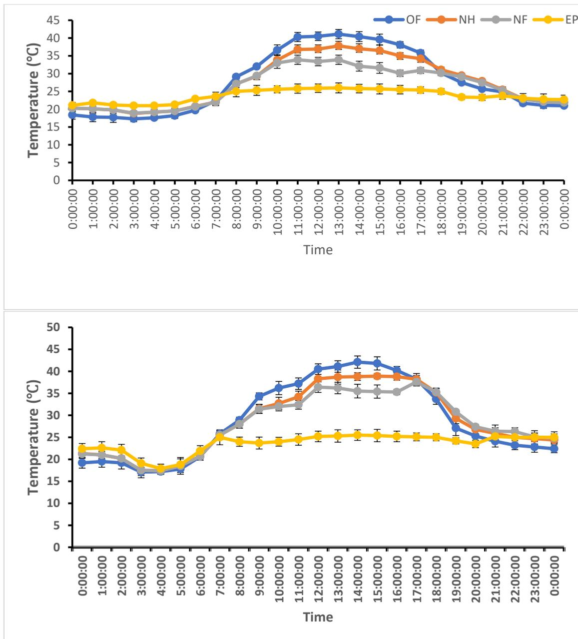
**Figure 2.** Hourly temperature changes during the peak of flowering and fruit set on 3 August 2020 (**upper figure**) and 5 August 2021 (**lower figure**) registered in the open field (OF), net house (NH), net house with fogging (NF, operating 6 S/36 S from 10 a.m. to 4 p.m.) and evaporative cooling under plastic house (EP). Standard error of the means was derived from three biological replicates.
