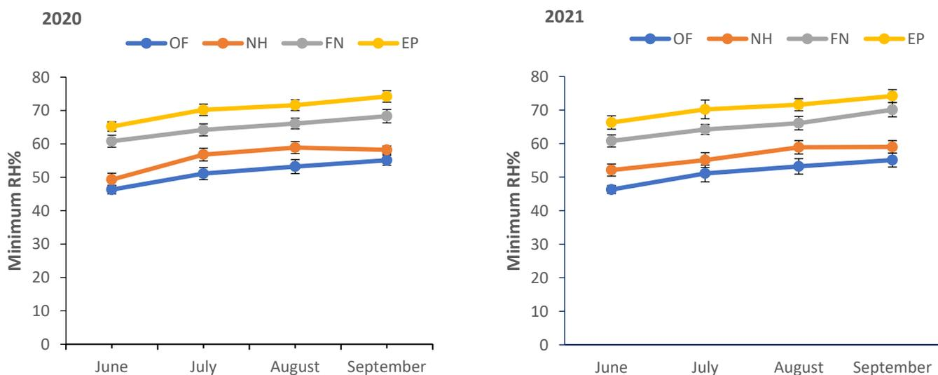
**Figure 7.** Average monthly minimum relative humidity percentage during the experimental periods of 2020 and 2021 seasons, registered in the open field (OF), net house (NH), net house with fogging (NF, operating 6 S/36 S from 10 a.m. to 4 p.m.) and evaporative cooling under plastic house (EP). Standard error of the means was derived from three biological replicates.
