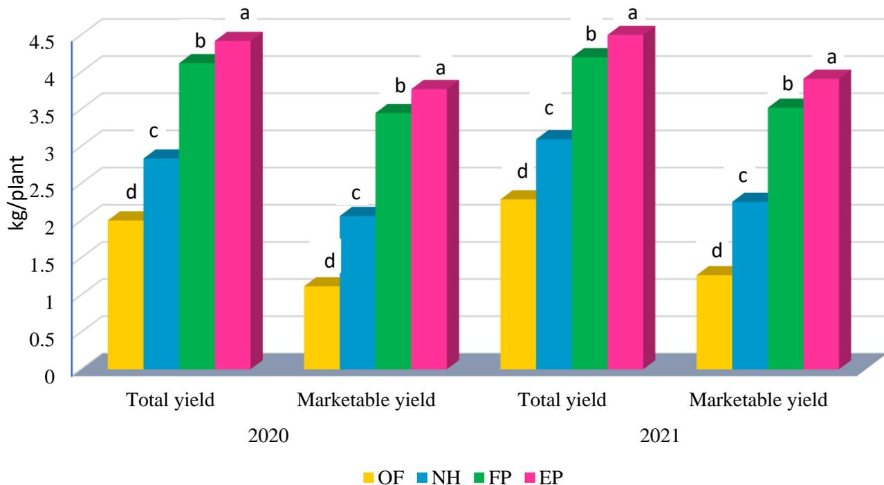
**Figure 10.** Total and marketable fruit yields of tomato in the open field (OF), net house (NH), net house with fogging (NF) operating 6 S/36 S from 10 a.m. to 4 p.m. and evaporative cooling under plastic house (EP). Different letters above the bars indicate that means are significantly different ( $p \leq 0.05$ ). Presented data are the mean of 3 biological replicates.
