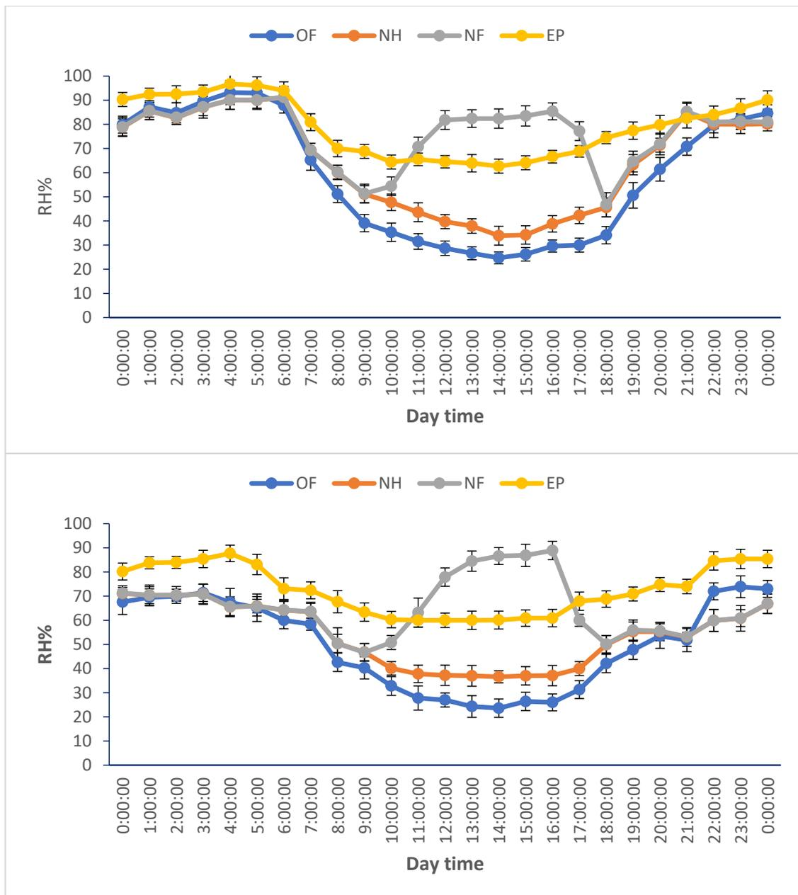
**Figure 3.** Hourly RH% changes during the peak of flowering and fruit set on 3 August 2020 (**upper figure**) and 5 August 2021 (**lower figure**) registered in the open field (OF), net house (NH), net house with fogging (NF, operating 6 S/36 S from 10 a.m. to 4 p.m.) and evaporative cooling under plastic house (EP). Standard error of the means was derived from three biological replicates.
