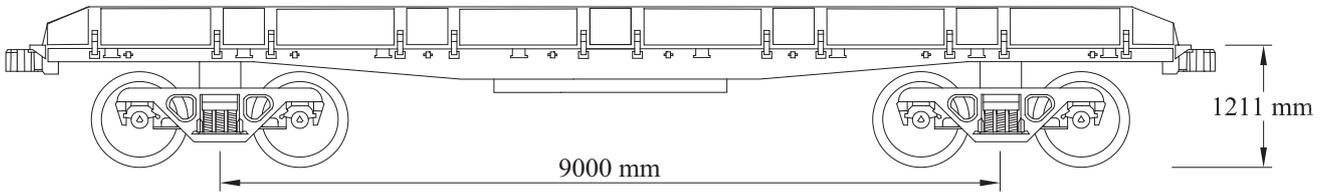
Fig. 9 Schematic diagram of N17 Wagon Flatcar.
