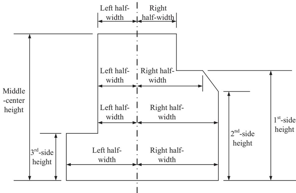
Fig. 1 Typical measures of widths and heights of a freight at an examined cross-section.
