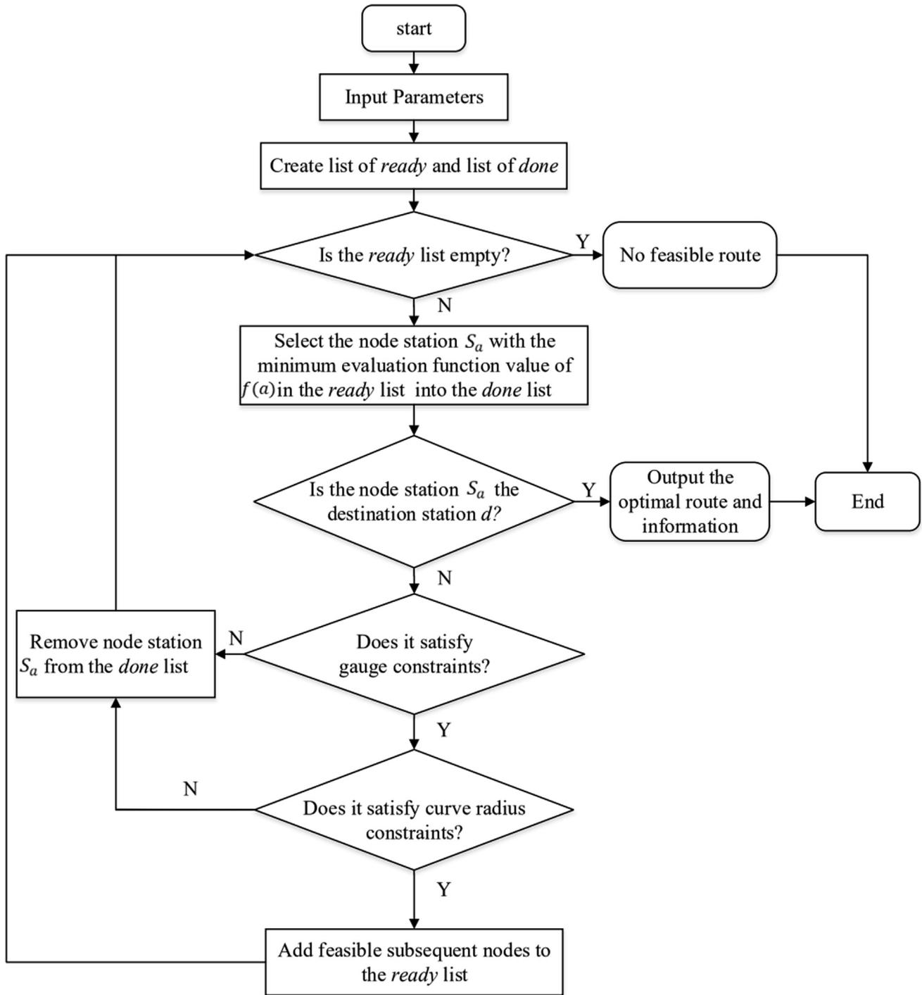
Fig. 8 Process of the proposed ROF-TRD.
