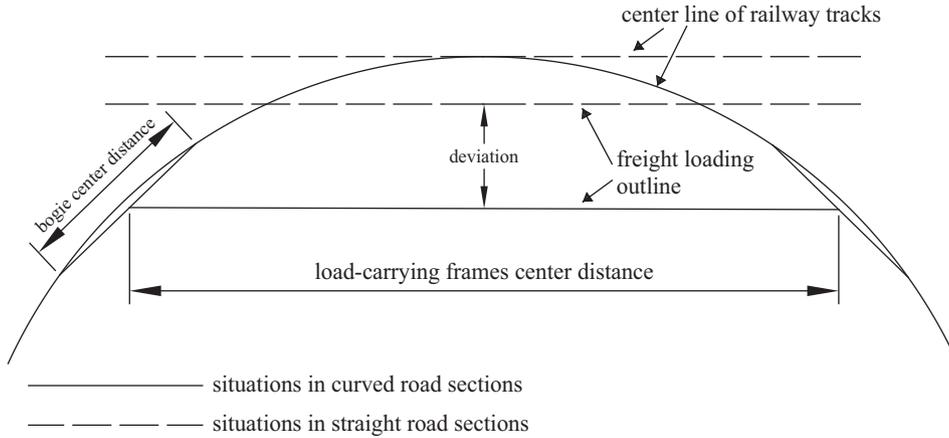
Fig. 14 Deviation of freight loading outline in curved road sections.
