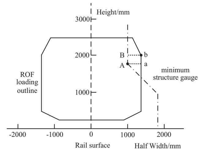
Fig. 6 Special positional relationship between gauge and ROF loading outline.
