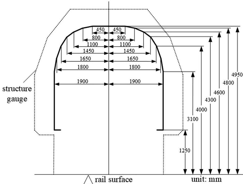
Fig. 5 Schematic diagram of out-of-gauge grades.
