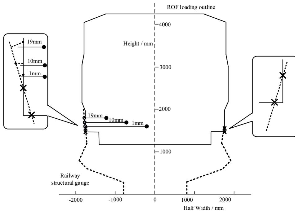
Fig. 12 Distances between railway structure gauges and ROF loading outline in the  $S_9$  to  $S_{9,d}^l$  interval section.
