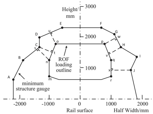
Fig. 2 Distances between freight loading outline and minimum structure gauge.
