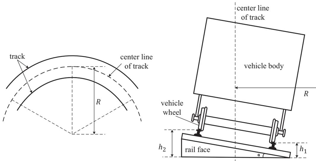
Fig. 3 The outer track superelevation in curved road section.
