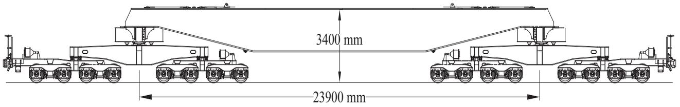
Fig. 13 Schematic diagram of D26B Wagon Well-Hole-Car.
