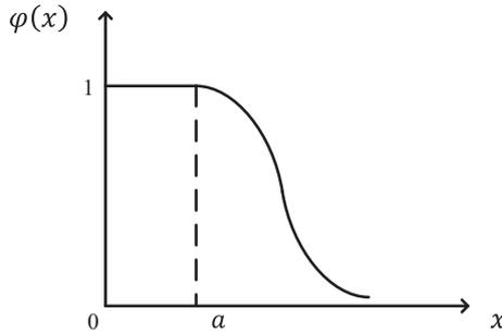
Fig. 4 Graph of distribution function of railway capacity loss.
