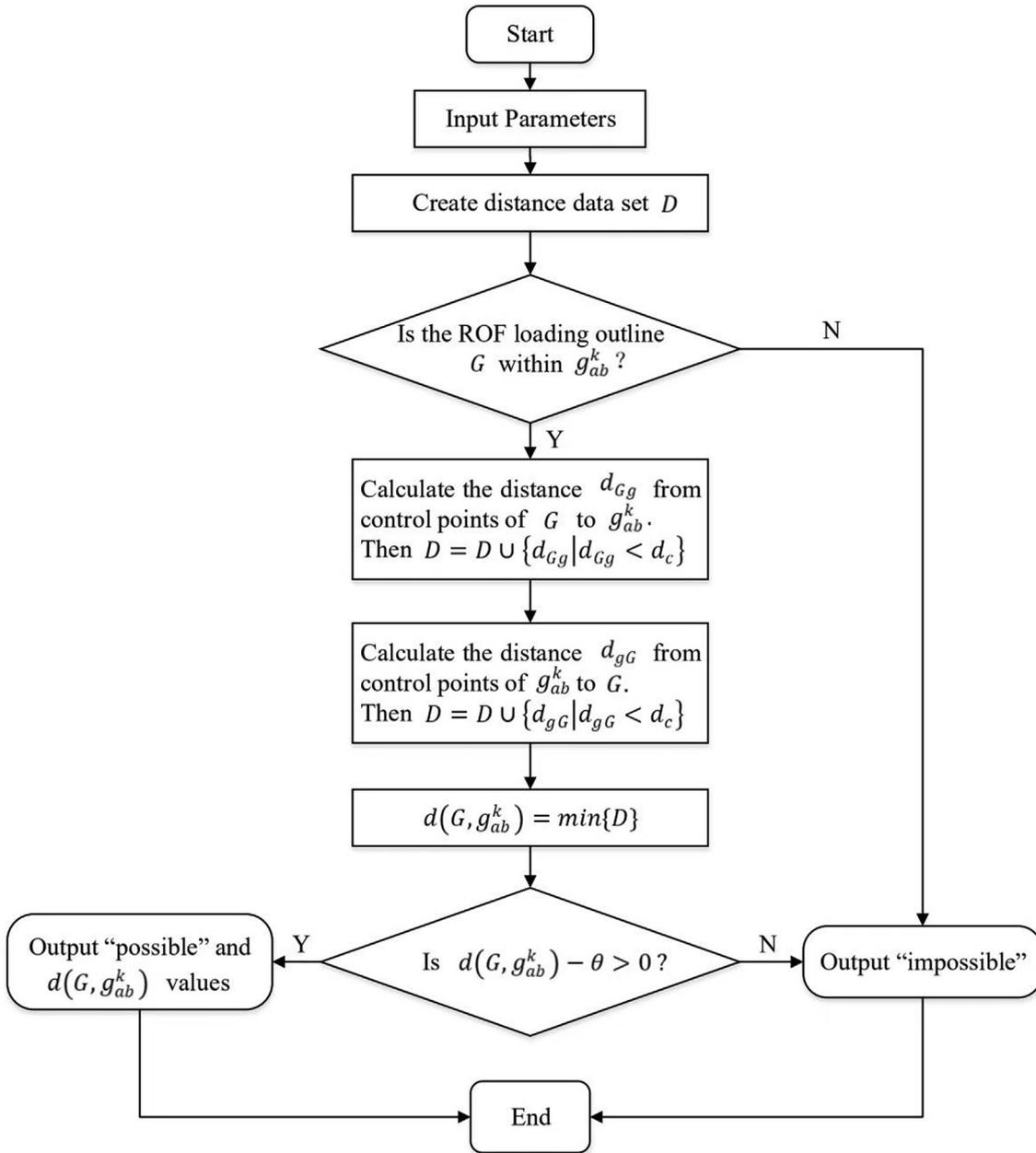
Fig. 7 Safety distance detection process.
