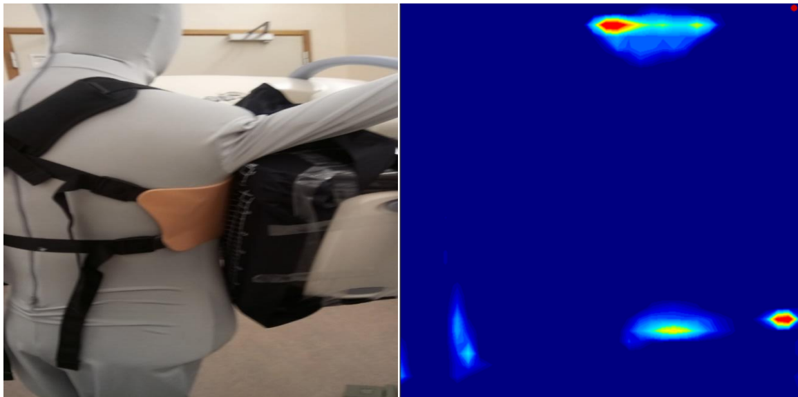
Figure 5.9 Phantom model positioned at IR angle 60° with the resultant contact pressure image.
