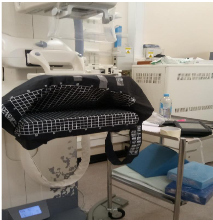
Figure 8.1 Xsensor pressure mat system wrapped around the IR and the paddle.
