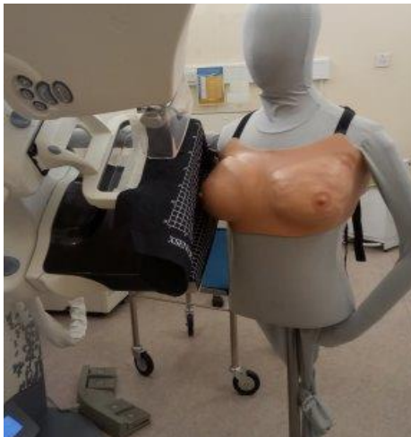
Figure 4.1 The Torso of the model mounted on a stand with breast phantom attachment.
