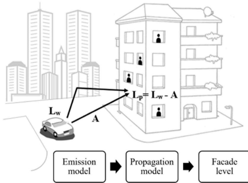
Fig. 1. Overall point-to-point prediction method.
