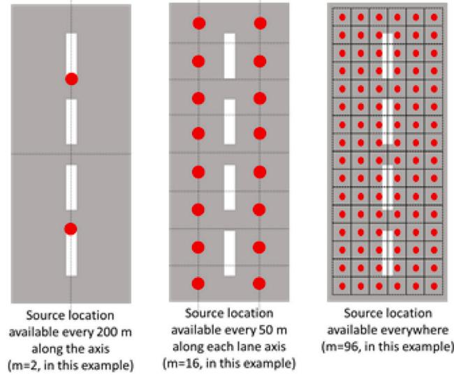
Fig. 2. Three plausible setups for defining the potential vehicle locations in a road segment.
