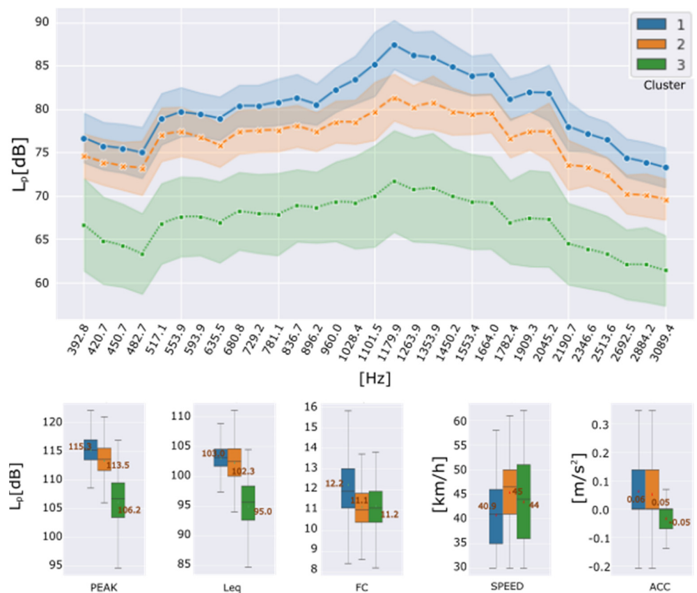
Figure 8. Urban avenue data clustering results. Features and driving conditions by formed clusters: Frequency domain (up); Peak level, Equivalent continuous sound level, Crest Factor, Speed and Acceleration (down).
