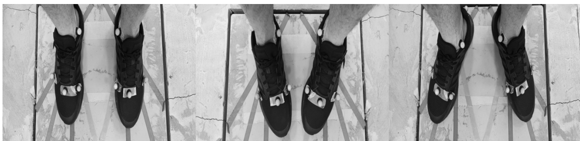
Figure 1: Feet placement over the force plate during the three static positions (Left picture = 0 degrees, Middle picture = Toe-in 20 degrees, Right picture = Toe-out 20 degrees)
