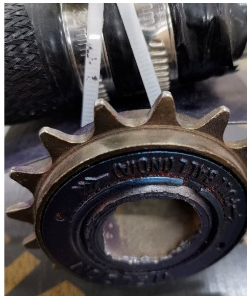
Figure 9. The freewheel to obtain unidirectional moving.
