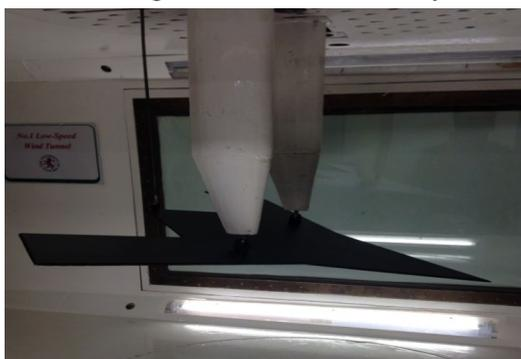
Fig. 3 - Flat plate flying wing configuration mounted in low-speed wind tunnel
