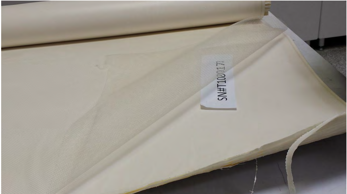
Figure 4-9. Membrane surface of the tail element and feed spacer during the autopsy.
