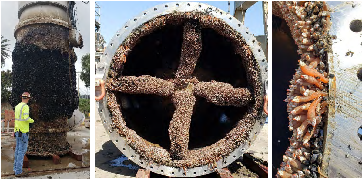
Figure 5-4. Biofouling at a 15.5 thousand m 3 /h submersible Brine dilution pump at CDP after one year of operation. Left: Pump body covered by mussels and barnacles. Middle: Pump discharge covered with barnacles. Right: Close-up of attached barnacles.
