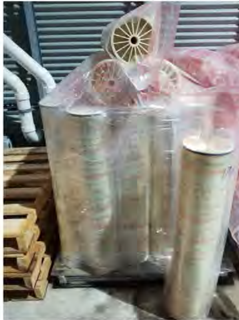
Figure 7: Pallet with membrane which need to be disposed.
