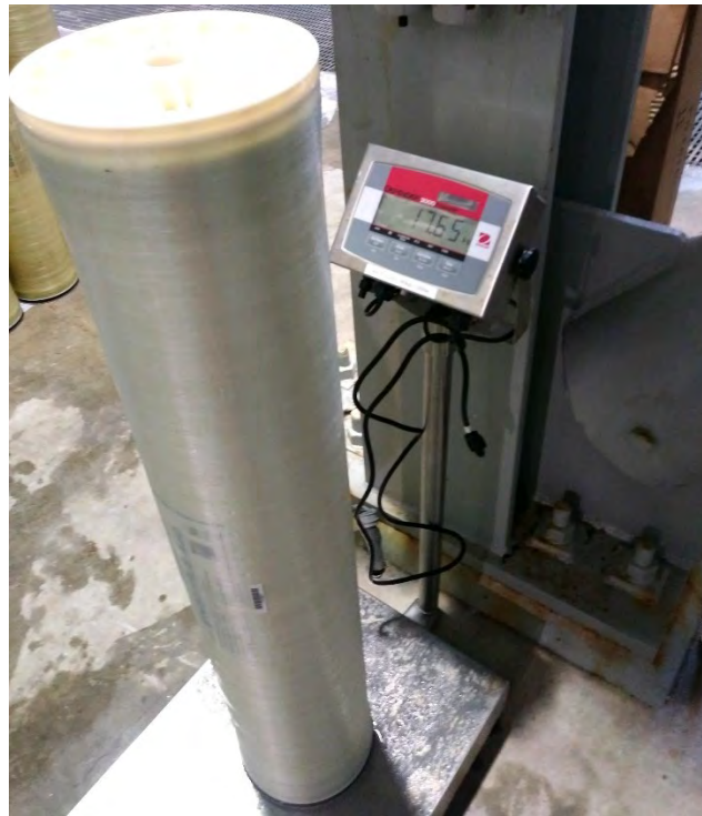
Figure 6-2. Inspection of biomass accumulation at the elements by weighting.
