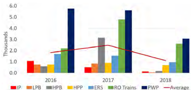
Figure 2-7. Total annual equipment downtime in hours.
