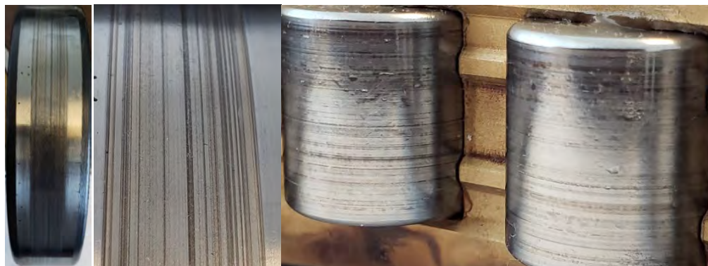
Figure 9-11: Left, Grooves inner raceway ring NDE bearing; Middle: expanded detail Grooves; Right, Denting roller surface.
