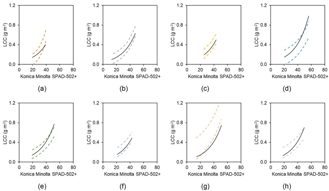
**Fig. C2.** Comparison of the generic Konica Minolta SPAD-502+ calibration function derived using all samples excluding oak (solid black line) against the 95% prediction intervals (dashed lines) associated with species-specific calibration functions for ash (a), beech (b), silver birch (c), hawthorn (d), hazel (e), red maple (f), oak (g), and sycamore (h).
