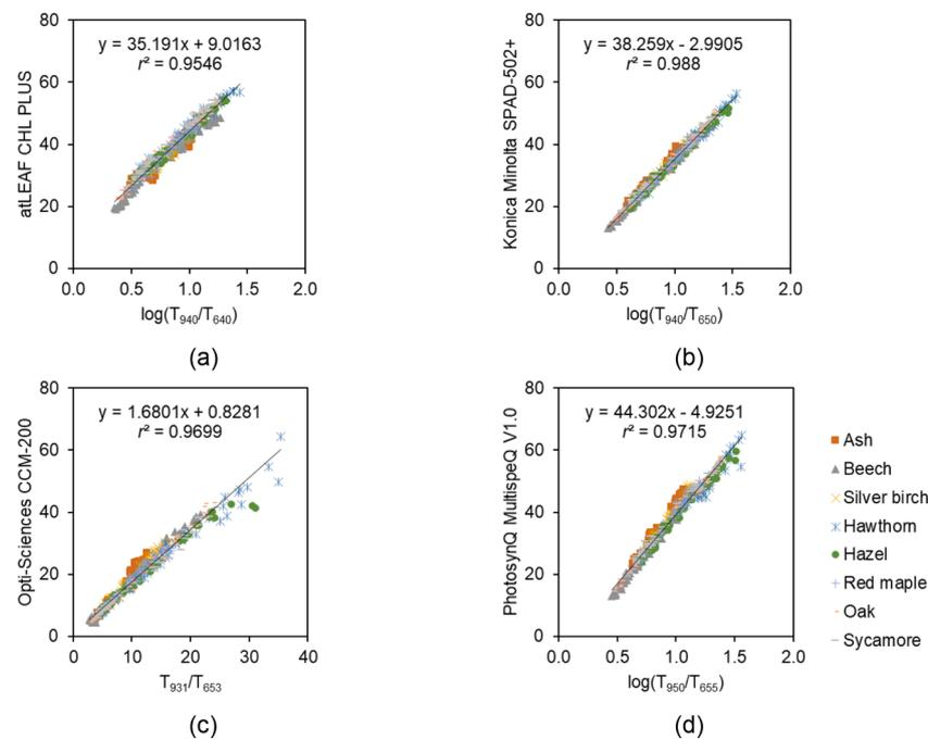
**Fig. 5.** Relationships between chlorophyll meter output values and transmittance-based indices representing the wavelengths and measurement equations of the atLEAF CHL PLUS (a), Konica Minolta SPAD-502+ (b), Opti-Sciences CCM-200 (c), and PhotosynQ MultispeQ V1.0 (d).
