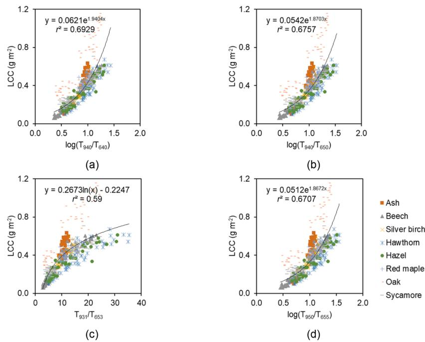
**Fig. 4.** Overall relationships between transmittance-based indices representing the wavelengths and measurement equations of the atLEAF CHL PLUS (a), Konica Minolta SPAD-502+ (b), Opti-Sciences CCM-200 (c), and PhotosynQ MultispeQ V1.0 (d) and destructively-determined LCC, for all investigated species.
