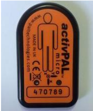
Figure 3.4: The activPAL™ micro accelerometer that was used in the study. The figure on the front indicates the correct orientation of the device to support correct application
