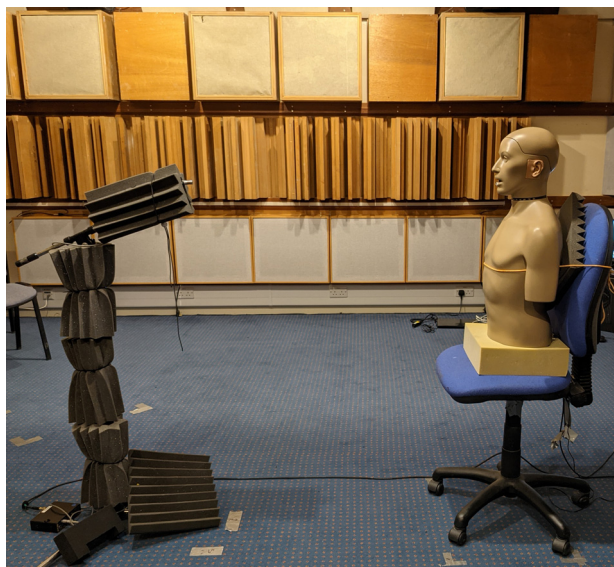
FIG. 1. (Color online) The measurement using the mannikin.
