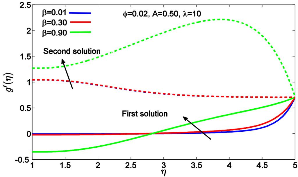
Fig 27: Effects of magnetic parameter ( $\beta$ ) on induced magnetic field profile for Mn-Zn nanoparticles when  $Pr = 6.2$  (Water),  $A = 0.5$ ,  $\varphi = 0.02$ ,  $\lambda = 10$ .
