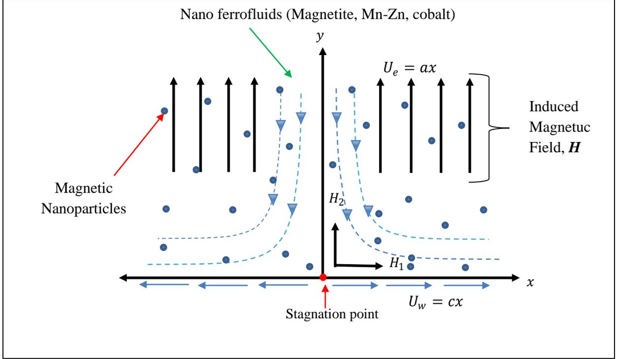
**Fig 1:** Schematic diagram of stagnation flow of nano-ferrofluid from a stretching sheet
