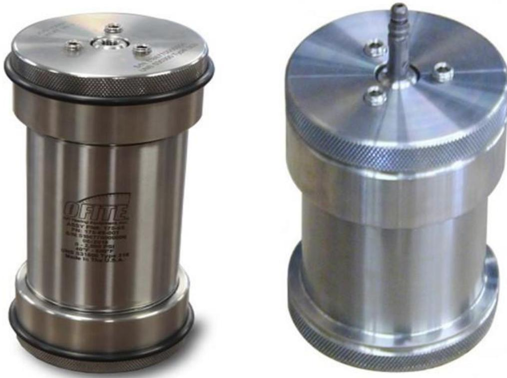
Figure 3.14: Aging cells, (LEFT) 500 ml, and (RIGHT) 260 ml [244]
