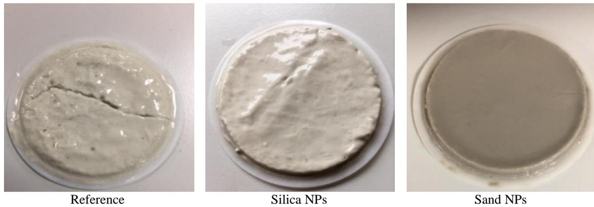
**Figure 4.18: Mud cake produced by mud containing nano silica and nano sand**
