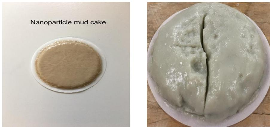
**Figure 4.6: Filter cake at HPHT conditions**
