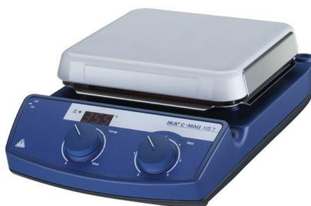
Figure 3.5: Magnetic plate stirrer
