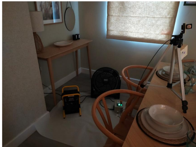
Figure 3.5 Examples of the co-heating test setup in the Zed House living room (top left), bedroom one (top right) and dining room (bottom)
