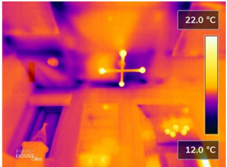
Figure 4.17 Thermography under no artificially induced pressure differential. Thermal inconsistency was observed on a region of the external wall (left) and across the first-floor ceiling (right).
