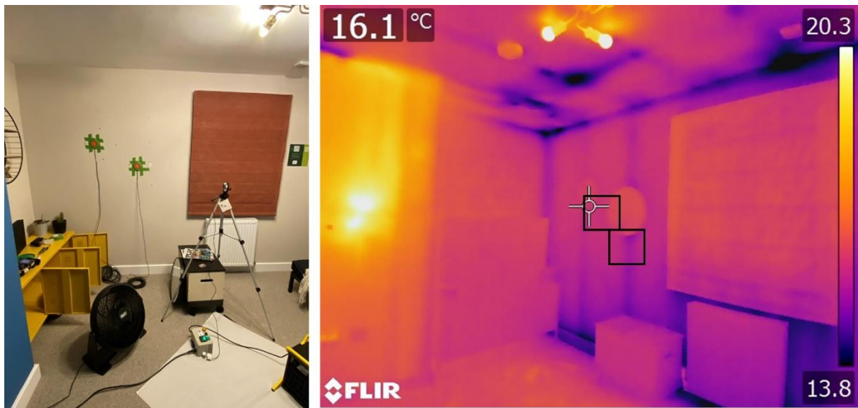
Figure 4.15 The locations of the two HFPs on the bedroom 3 wall. Unfortunately, the thermal image was taken after the removal of the HFPs
