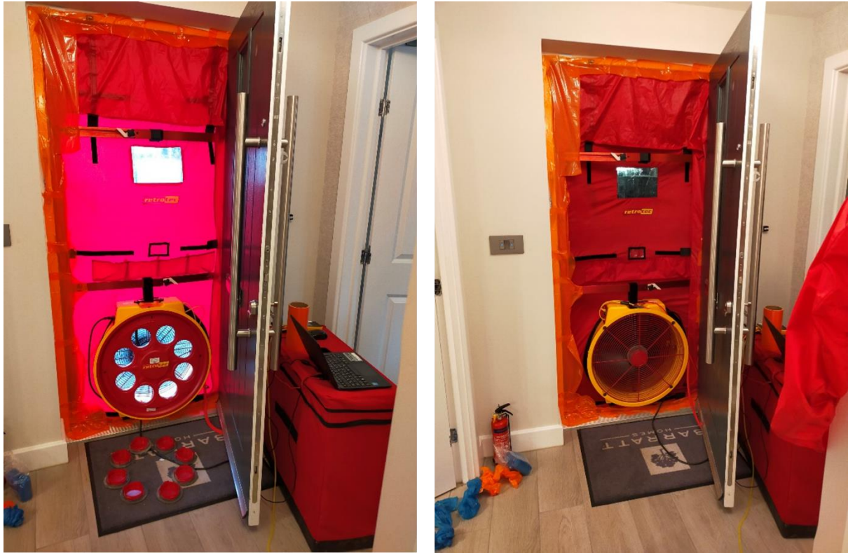
Figure 3.6 The blower door test setup in the Zed House ready for depressurisation (left) and pressurisation (right)
