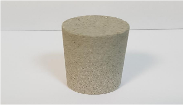
Figure 3.12: Berea Lower sandstone 1"x 2" size photographic image
