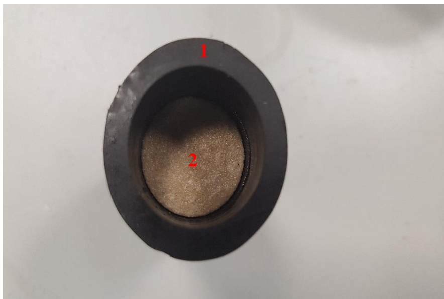
Figure 3.24: 1"x 2" Core sample sleeve (top view)
