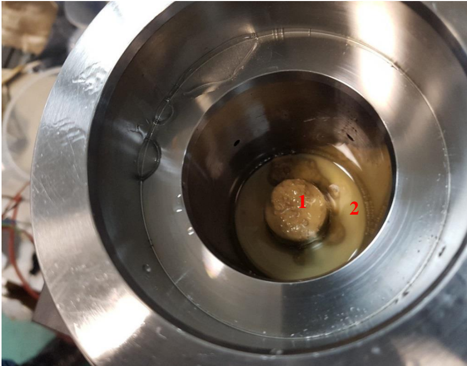
1 Sludge on distribution plug 2 Overburden oil
