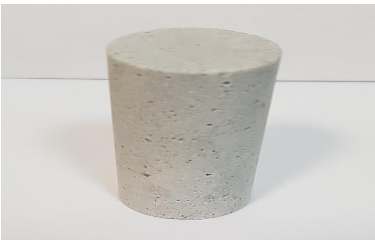
Figure 3.13: Silurian dolomite (Carbonate) 1"x 2" size photographic image
