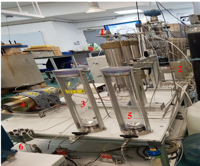
Figure 3.32: Core flooding injection cells and acoustic core holder assembly
