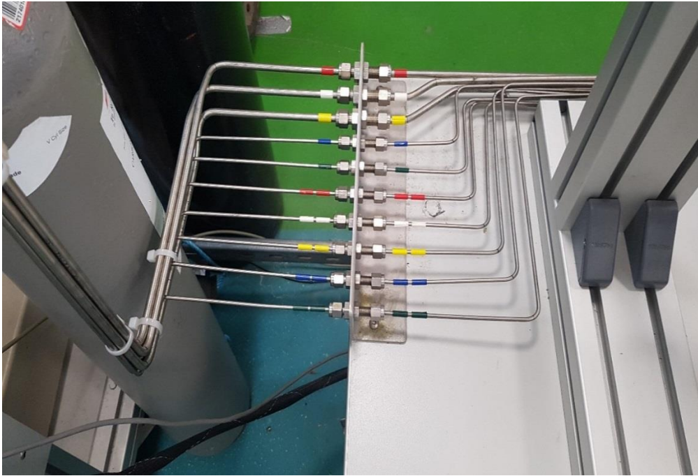
Figure 3.30: Core holder flowlines to pressure transducers
