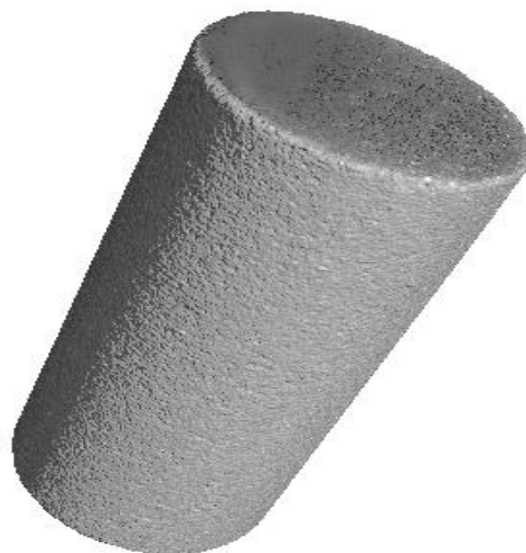
Figure 4.22: CT volume reconstruction of Grey Berea at Transparency setting of 200
