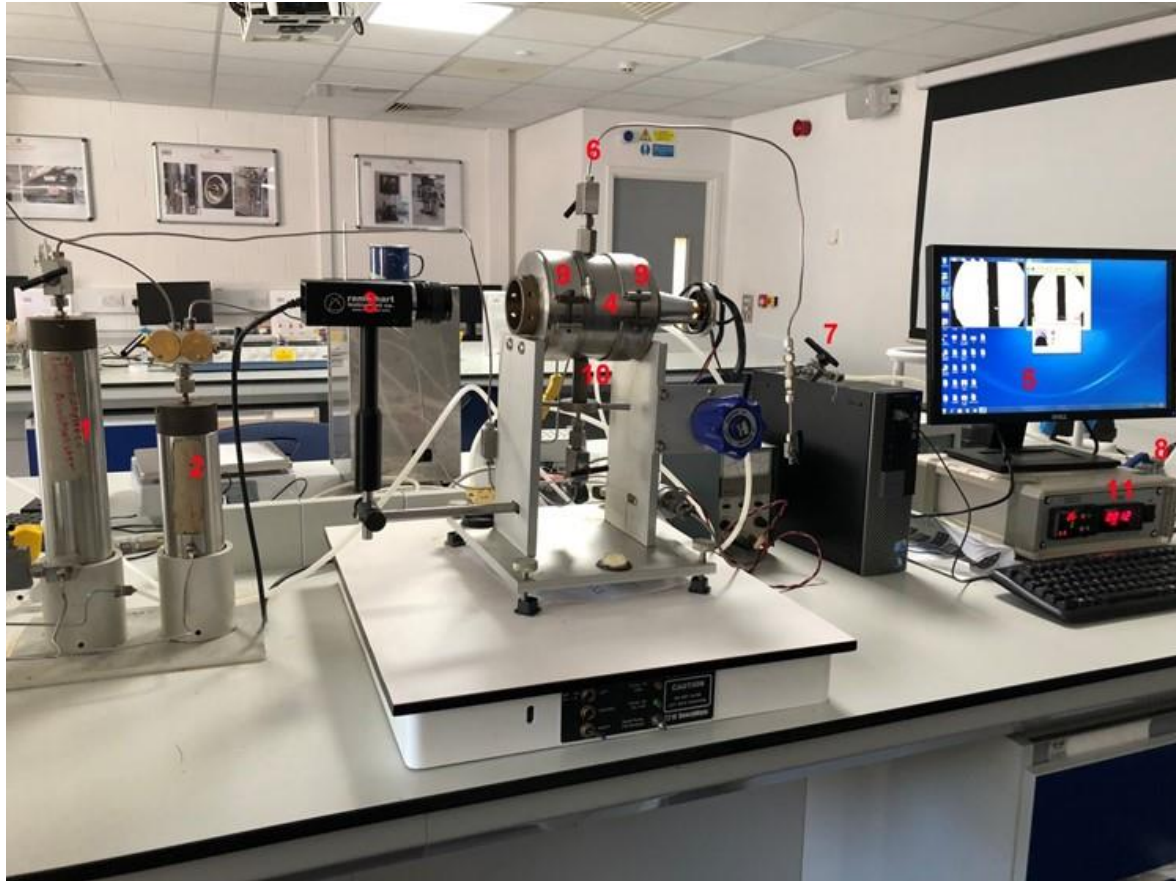
(1&2) accumulators, (3) Rame hart digital camera, (4) IFT cell, (5) Monitor, (6) Vent Valve, (7) Vacuum Valve, (8) Vacuum pump, (9) Heating element, (10) Injection Needle, (11) data logger and temperature controller
