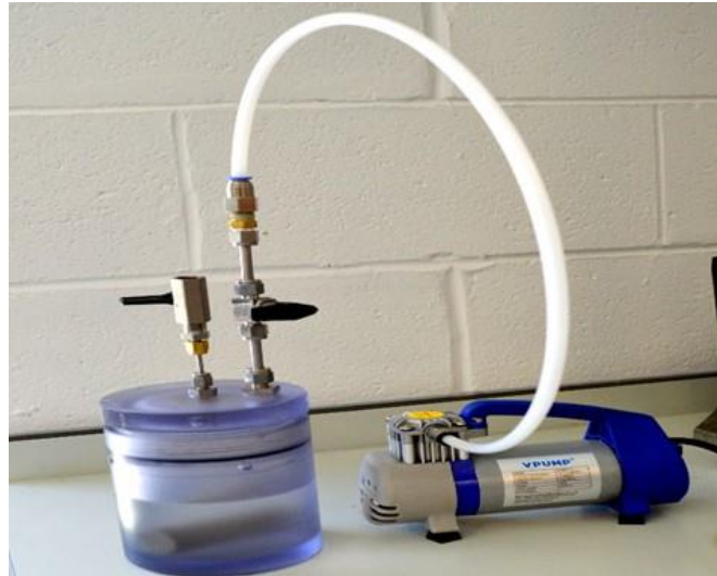
Figure 3.11: Vacuum Pump for Saturation Method
