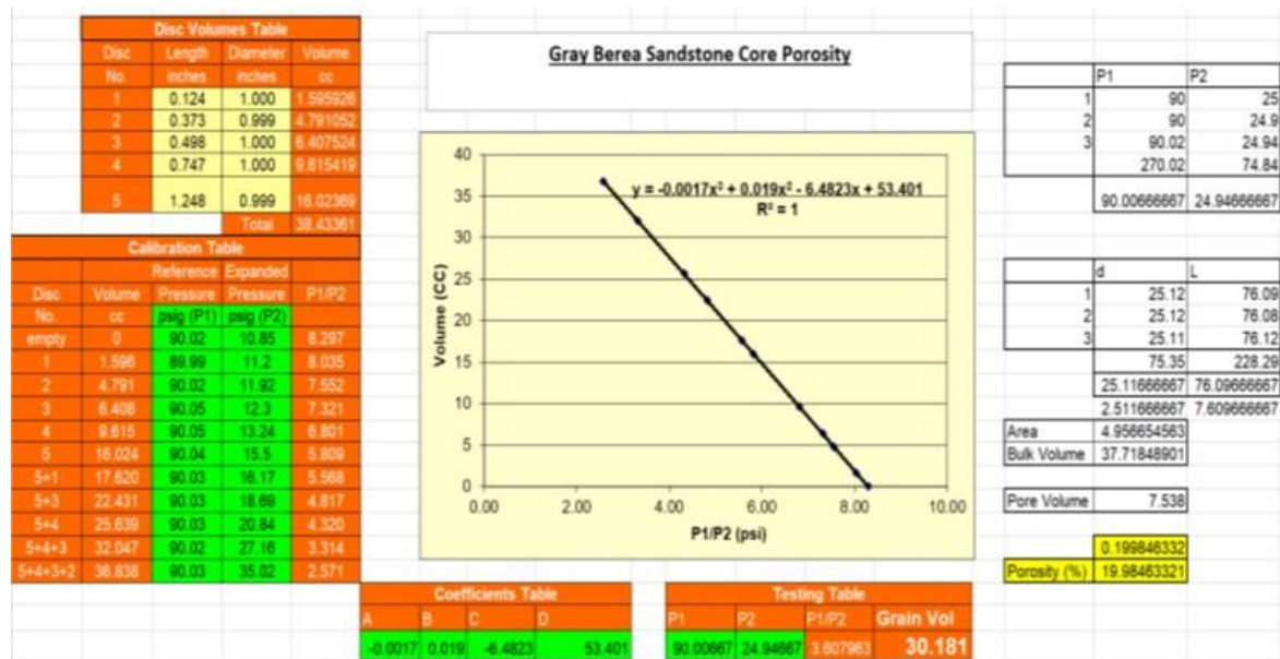
Figure 3.10: Excel Spreadsheet for Porosity Determination using Helium Porosimeter
