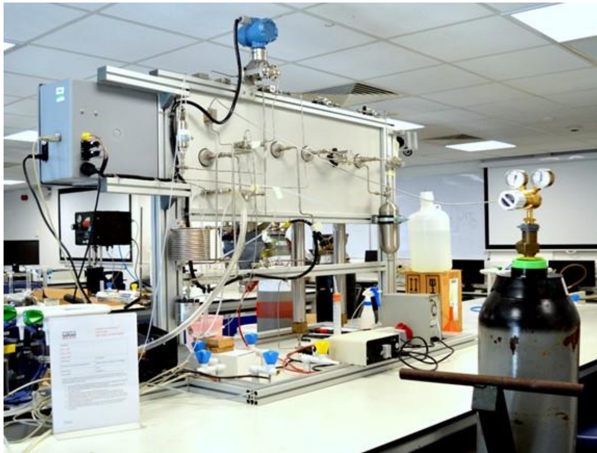
Figure 3.12: PREL-300TM Core Flooding Setup (Front and Back View)
