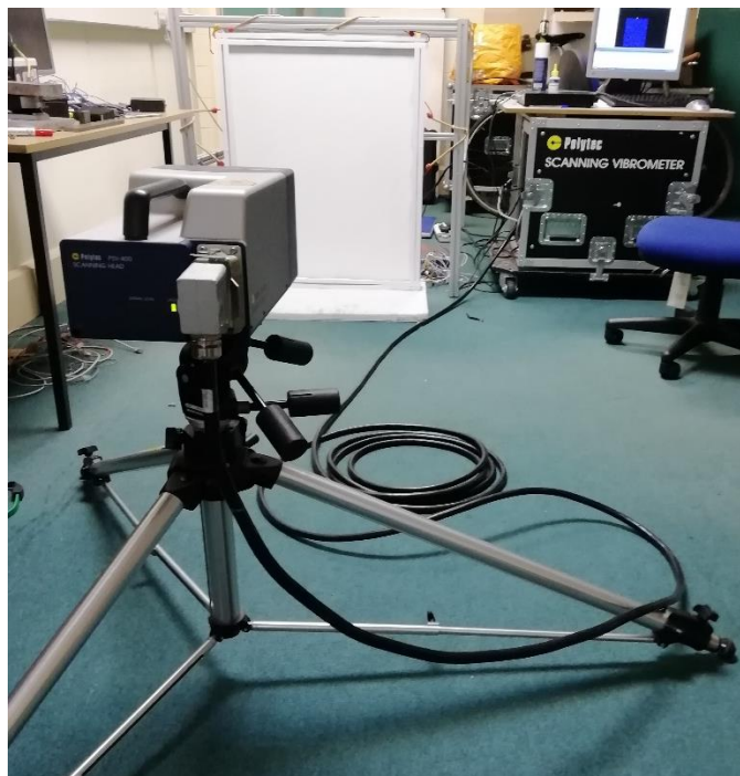
Figure 3.17: PSV 400 scanning laser vibrometer in-situ for plate experiment detailed in Chapter 6
