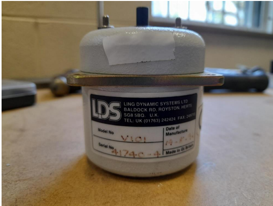
Figure 3.24: Bruel & Kjaer LDS V101 permanent magnet shaker
