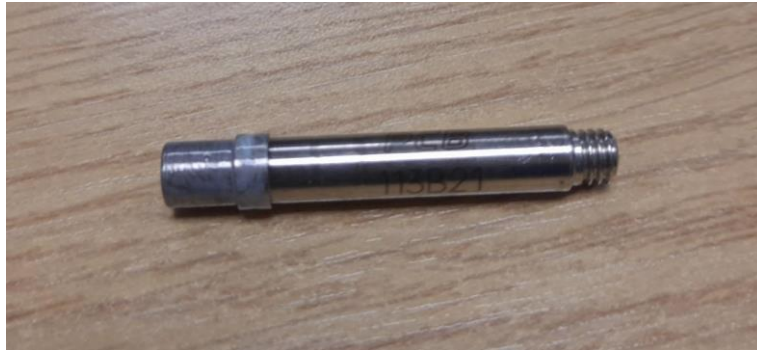
Figure 3.2: PCB piezoelectronics 113B21 pressure transducer
