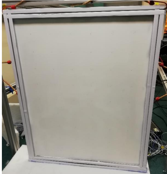
Figure 3.29: Plate mounted in-situ. The surface of the plate has been coated with a non-metallic matte white paint in order to reduce reflections, allowing the laser to take clearer measurements.
