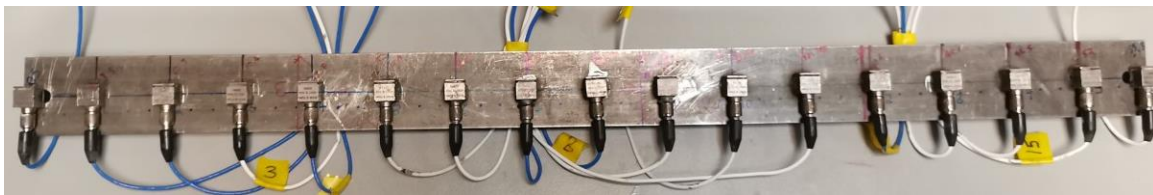
Figure 3.27: Experimental steel beam. 17 accelerometers are mounted on the bottom side of the beam at interval of 3.2cm. The beam was excited using an instrumented force hammer at each of the same positions on the upper face of the beam.
