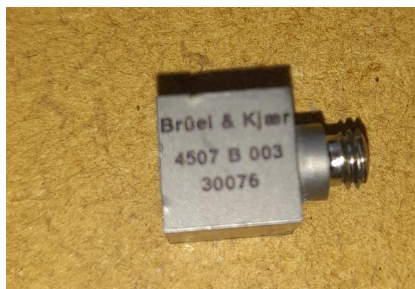
Figure 3.22: Bruel & kjaer Type 4507 accelerometer
