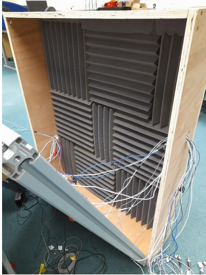
Figure 3.33: Interior of plate baffle showing acoustic foam
