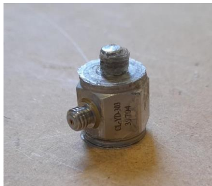
Figure 3.23: Sinocera CL-YD-303 2kN Compression only force transducer
