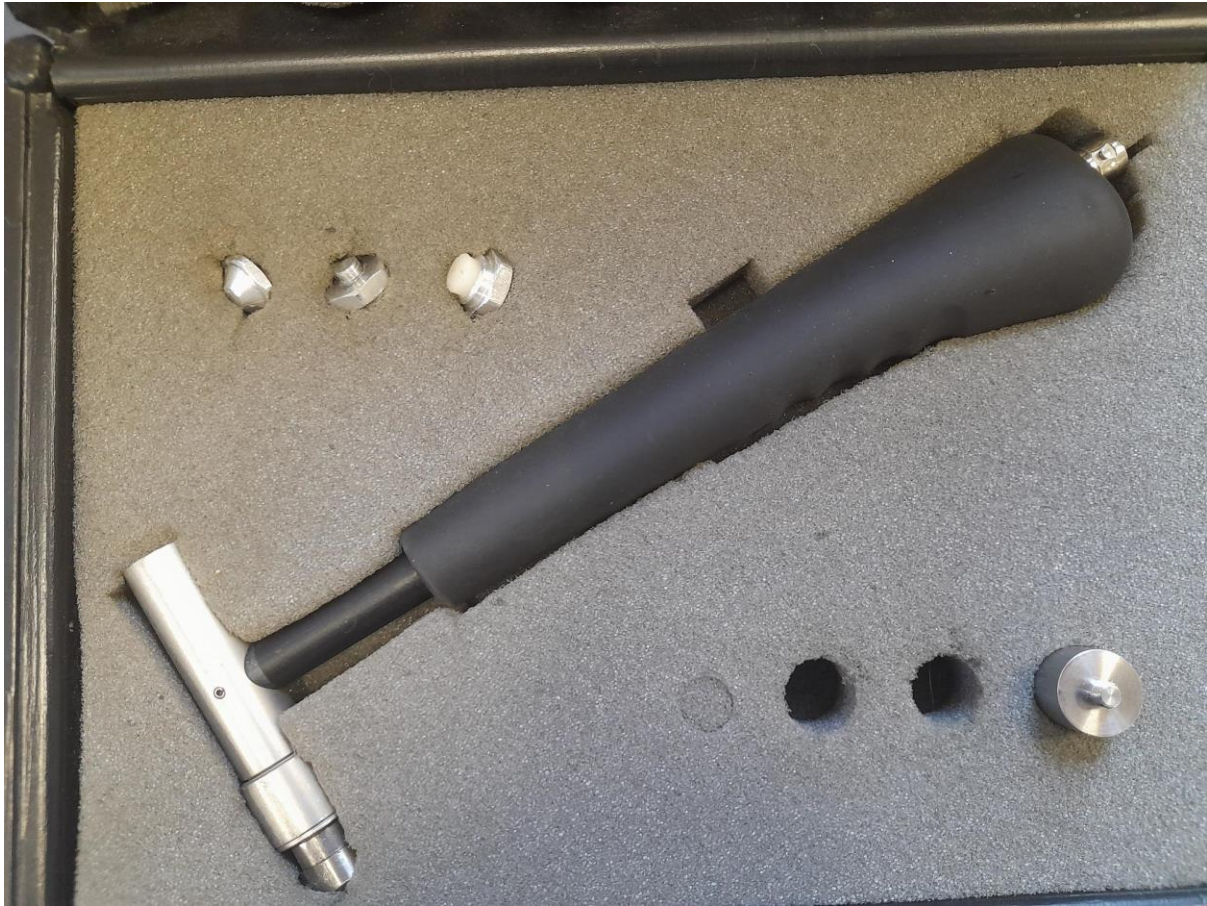
Figure 3.21: Impact hammer in case with tips shown in upper left of photograph. The left tip is the metal tip, the middle shows the side which is screwed into the hammer of another metal tip, and the right tip is the plastic tip. The bottom right element is a weight or extender which can be added to the hammer.
