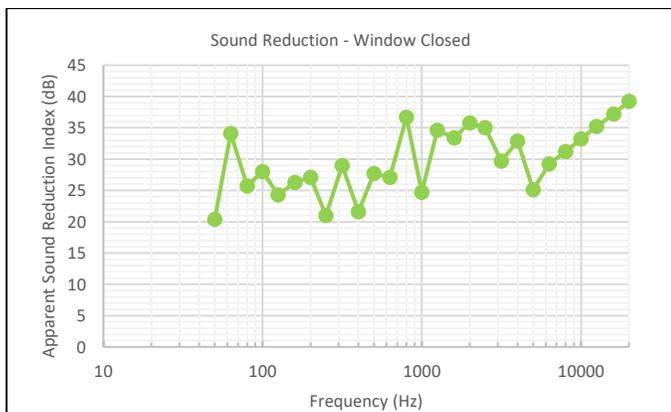
Figure 11. Third Octave Sound Reduction Values – Closed Window
