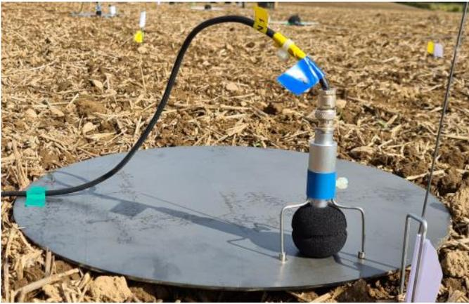
Figure 2. Inverted microphone tripod, mounted onto ground plate with wind shield
