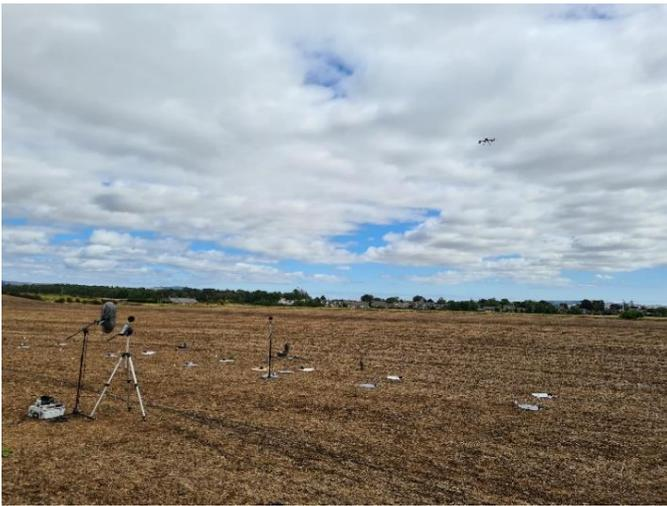
Figure 6. Photograph of the measurement set up recording measurements of the DJI Matrice 300 (M3)
