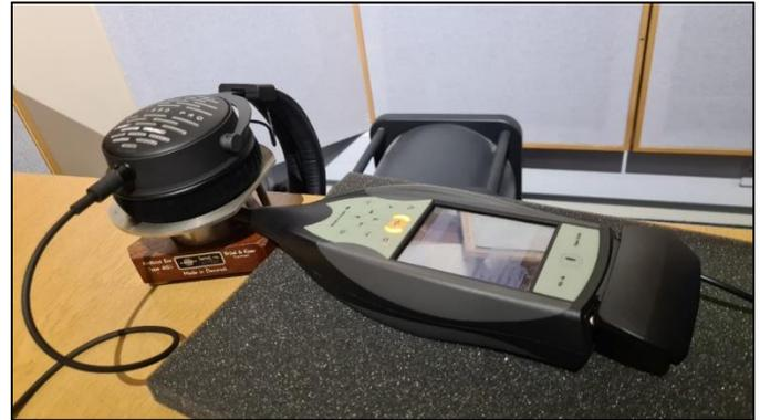
Figure 12. Sound Level Meter and Artificial Ear Being Used for Calibration
