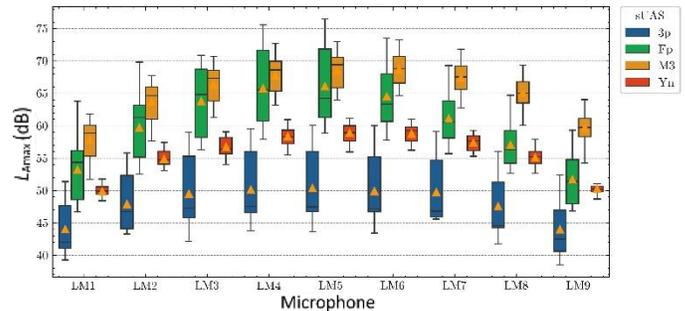
Figure 8.  $L_{Amax}$  data measured at each of the microphone positions for each of the four UAS
