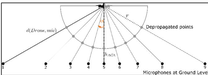
Figure 4. Ground microphone positions for lateral directivity resolution and depropagated points, illustrating how de-propagated drone noise distances will be defined
