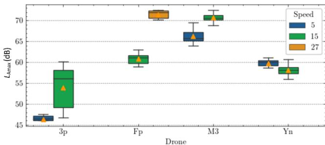
Figure 7.  $L_{Amax}$  measured at centre microphone for each of the four UAS and flight speeds (m/s)
