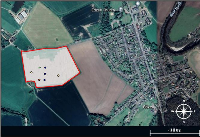
Figure 1. Satellite imagery showing measurement location. Blue dots indicate microphone array (centre point and outer limits), yellow dots the UAV flight path, green dot the meteorological station and orange where background measurements were taken
