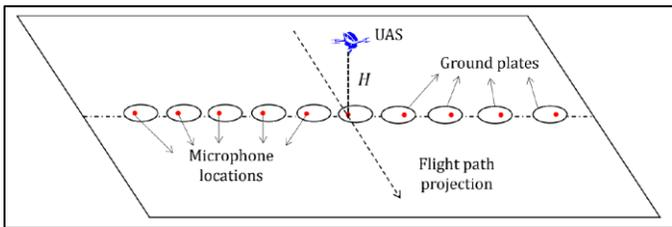
Figure 3. Schematic showing the microphone orientation and positions relative to the UAS flight path [2]
