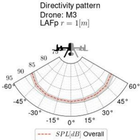
Figure 9. 2D directivity data of the broadband sound pressure level from the Matrice 300 (M3) backpropagated to 1m distance from the UAS
