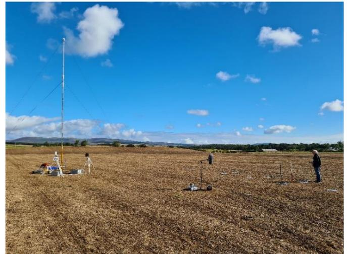
Figure 5. Photograph of the measurement set up. Left: 10m Meteorological mast, Centre right: Ambisonic microphone position, Right: ground plate microphone array
