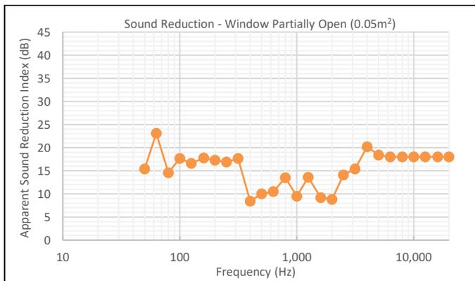
Figure 10. Third Octave Sound Reduction Values – Partially Open Window
