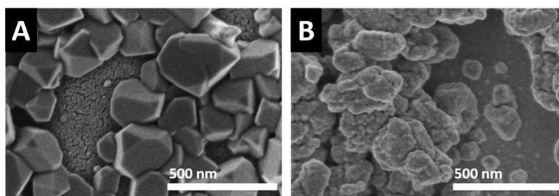
**Figure 4.** SEM images of electrodeposited copper on an Au-coated  $\text{Si}_3\text{N}_4$  membrane (A) before  $\text{CO}_2$ RR and (B) after  $\text{CO}_2$ RR ( $-1.8$  V vs Ag/AgCl in 100 mM  $\text{KHCO}_3$  saturated with  $\text{CO}_2$ ).
