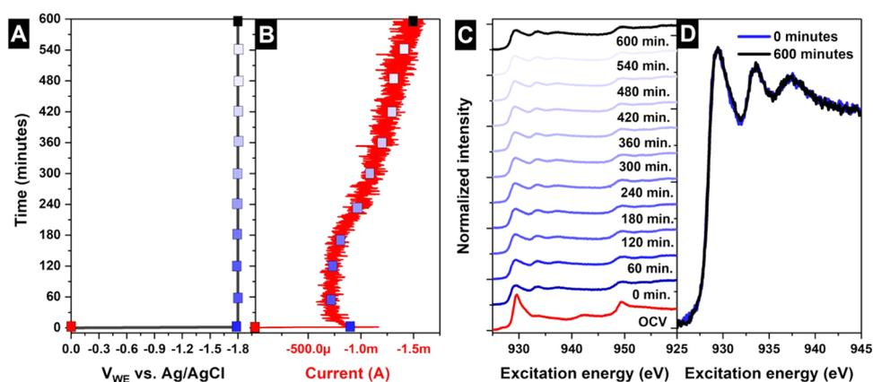
**Figure 3.** (A) Applied voltage, (B) current, and (C) Cu  $L_{2,3}$  edges in FY mode depending on the time at  $-1.8$  V vs Ag/AgCl (under  $\text{CO}_2$ RR conditions) in the presence of 100 mM  $\text{KHCO}_3$  saturated with  $\text{CO}_2$ . (D) Cu  $L_3$  edge in FY mode depending on the time at  $-1.8$  V vs Ag/AgCl (under  $\text{CO}_2$ RR conditions) in the presence of 100 mM  $\text{KHCO}_3$  saturated with  $\text{CO}_2$ .
