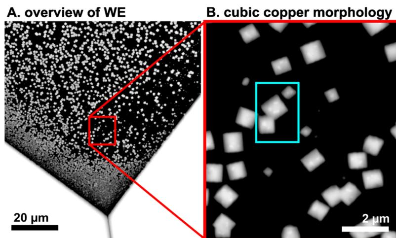
**Figure 5.** *In situ* EC-SEM images of fresh electrodeposited copper in OCV conditions using a large field: (A) overview of the transparent window exemplifying the homogeneous distribution of the material at the electrode and (B) a close-up look revealing the cubic structure of electrodeposited copper.
