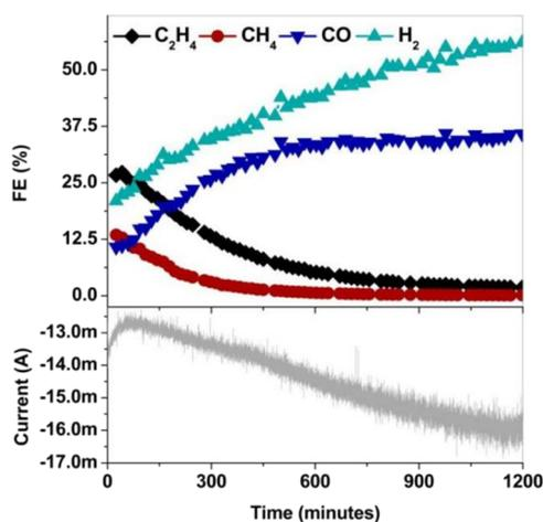
**Figure 1.** Top: gaseous product distribution of the  $\text{CO}_2\text{RR}$  reaction (in  $\text{CO}_2$ -saturated 100 mM  $\text{KHCO}_3$  at  $-1.8 \text{ V vs Ag/AgCl}$ ) over an electrodeposited copper electrode on gold as a function of time. Bottom: Total cathodic current over time collected in an H-type electrochemical cell (see the [Experimental Section](#)).
