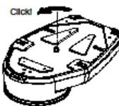
1. Turn the locking pin on the base of the housing a quarter-turn anticlockwise.
