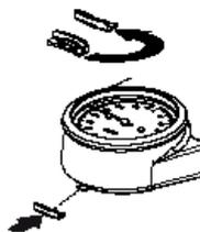
1. Position the transport lock as shown in the adjacent drawing.
