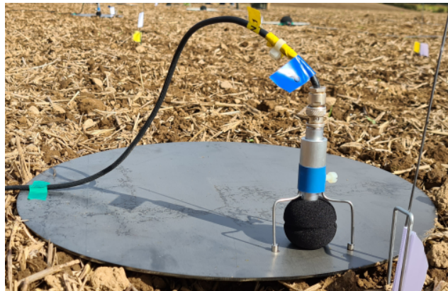
(a) Ground Microphone setup, accordingly to ICAO [50].
