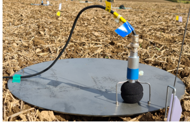
(a) Ground Microphone setup, accordingly to ICAO [50].
