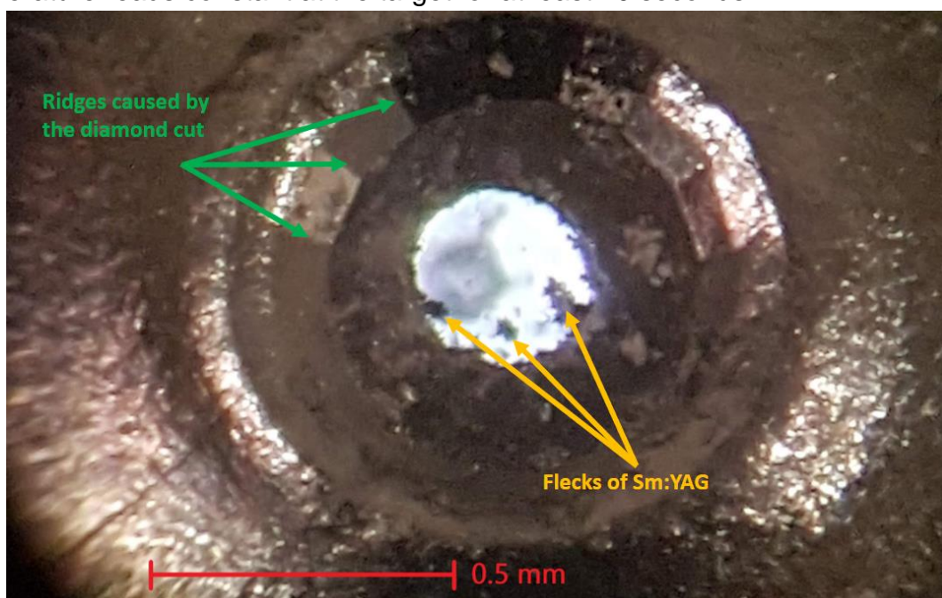
Figure.6: A photograph of a prepared gasket, taken through a 20x magnification microscope. The flat indented surface is 0.6mm in diameter, matching the diamond culet that formed it. Note the ridges in the indentation walls, caused by the cut of the diamond. The small dark flecks in the bottom-left, bottom-middle and larger fleck at bottom-right of the hole are small shards of pressure scale crystal, in this case Sm:YAG, positioned away from the centre to be easily avoided when taking nitrogen Raman spectra. The larger, slightly lighter mark in the middle-left of the hole is simply dirt on the back of the diamond and is out of focus when readings are taken. The impact of such contaminants is mostly negligible.
