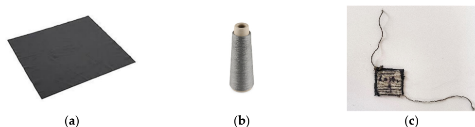
Figure 3. Materials used for sensor development: (a) conductive stretchable fabric, (b) silver-plated conductive thread, (c) designed sensor.
