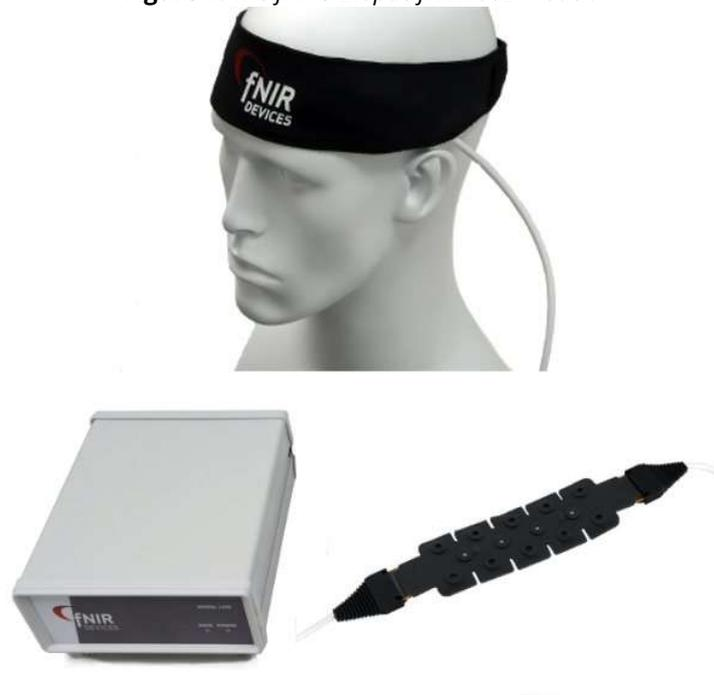
*Note.* This figure shows the hardware utilised to collect the level of HbO on the PFC of the subject. The box was connected to a computer loaded with Cognitive Optical Brain Imaging studio (COBI) software. Photo Courtesy of ©BIOPAC Systems, Inc.
