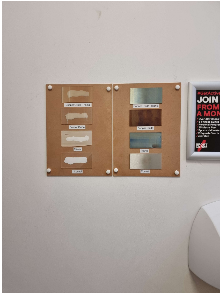
Figure 3.1: In-situ photograph of surfaces placed in the gender neutral toilets, mounted vertically to the wall. Surfaces were mounted to the back boards using a strong adhesive paste, and were mounted near a hand drying vent.
