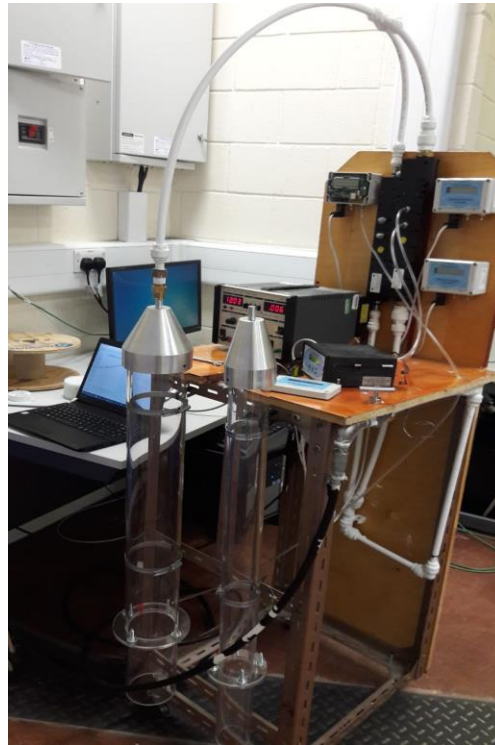
Figure 3.7.: Airflow resistivity test setup at University of Salford laboratory
