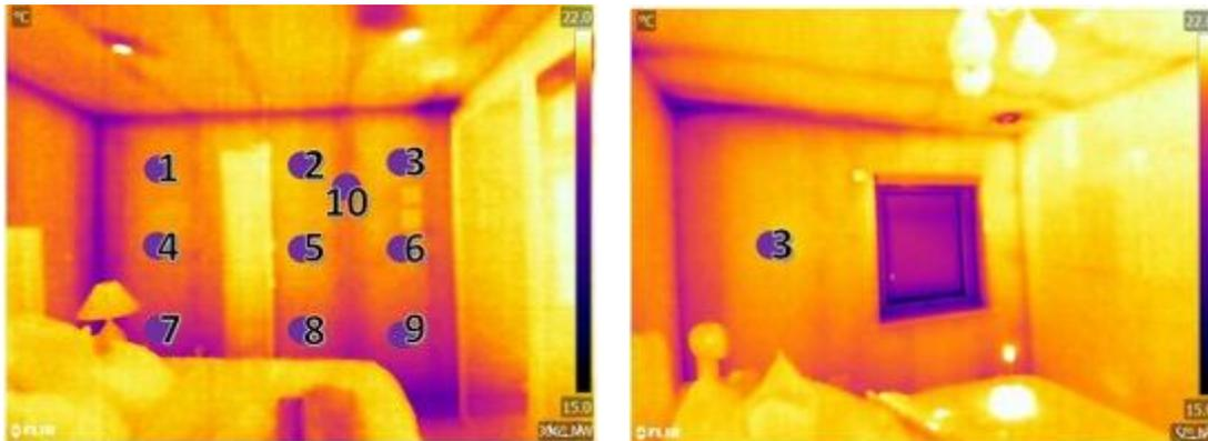
Figure 41. Thermogram showing locations of external wall in-situ U-value measurements.
