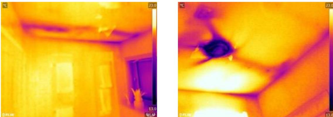
Figure 22. Bathroom at atmospheric pressure (left), cold spots indicating gaps in the loft insulation placement. During depressurisation (right) air infiltration visible along the ceiling particularly at penetrations.
