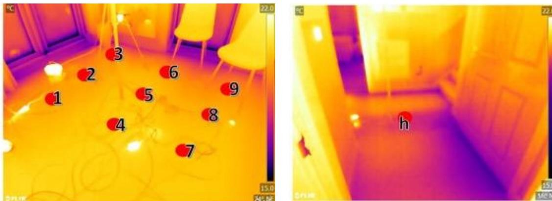
Figure 43. Thermogram showing locations of floor in-situ U-value measurements (a) Kitchen (b) Hall.
