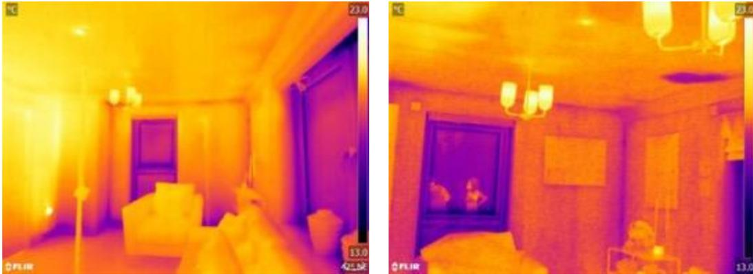
Figure 24. Living Room atmospheric pressure (left). During depressurisation (right) air infiltration visible along the ceiling, floor and vents. Particularly cold spot under depressurisation stemming from the inter-floor void, further investigation required to understand the cause.
