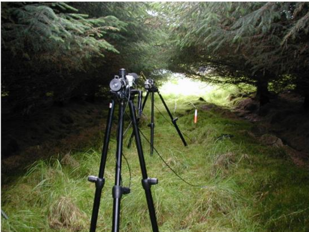
Figure 33 - ANSI S1.18-1999 excess attenuation spectra measurements at 2 of the locations during Spadeadam 2002 field trials (Waddington, 2002).
