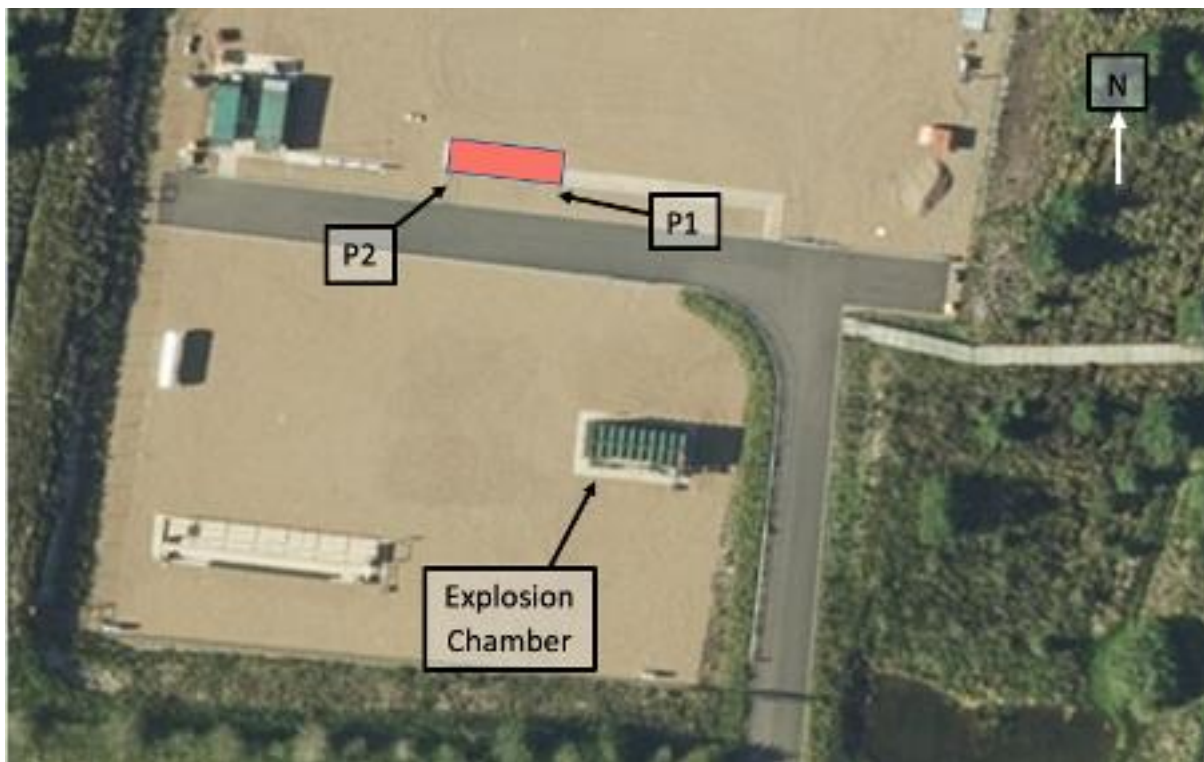
Figure 12 - Measurement locations during the August 2020 trials. P1 and P2 (location of pressure gauge) are representative of the worst-case personnel positions. The red coloured area represents the area that personnel will be present during hazard awareness demonstrations.
