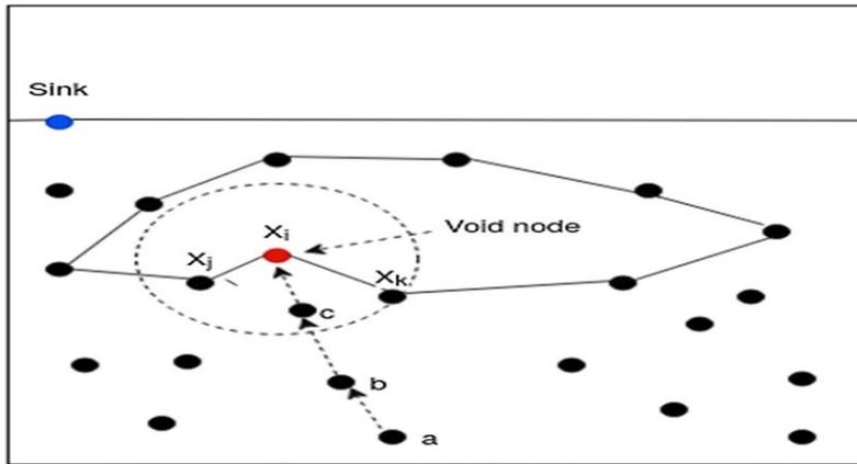
Figure 3.13: Network model for void and trap nodes (Source: Nazareth & Chandavarkar, 2022)
