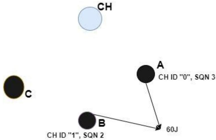
Figure 5.19: Scenario for the selection of eligible cluster head in subsequent round using SFV (1)
