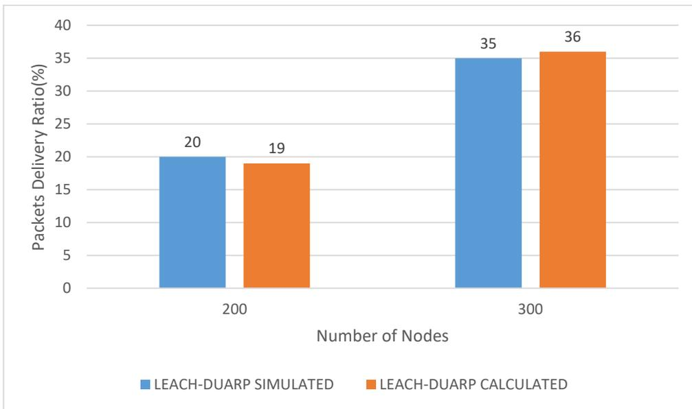
Figure 7.6: Comparison for packet delivery ratio for LEACH-DUARP
