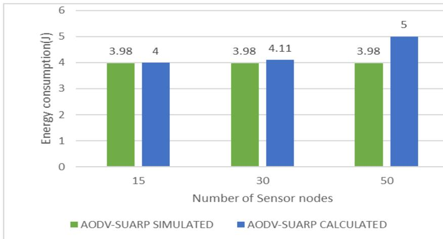
Figure 7.1: Comparison of simulated and calculated energy consumption of AODV-SUARP
