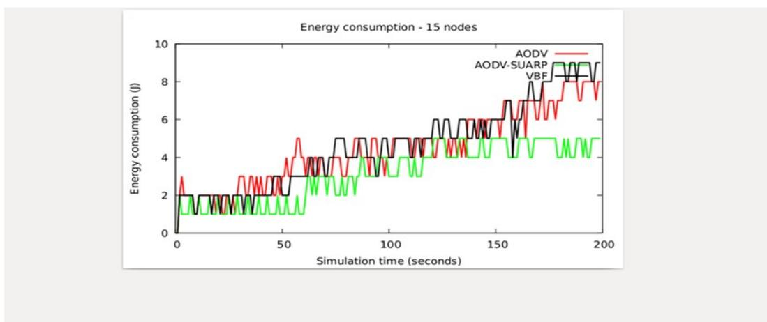
Figure 6.7: Energy consumption for 15 nodes
