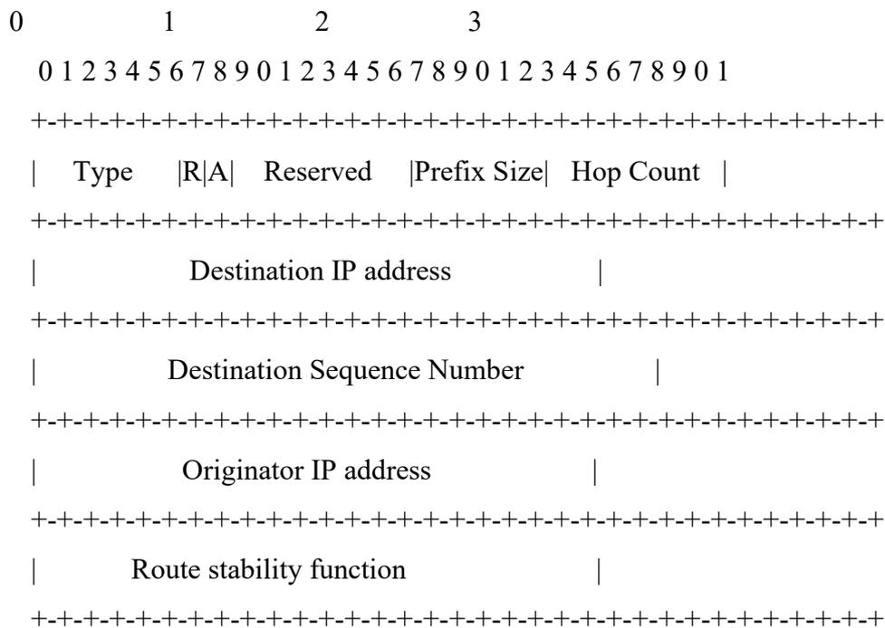
Figure 5.10 Route response message format for AODV-SUARP
