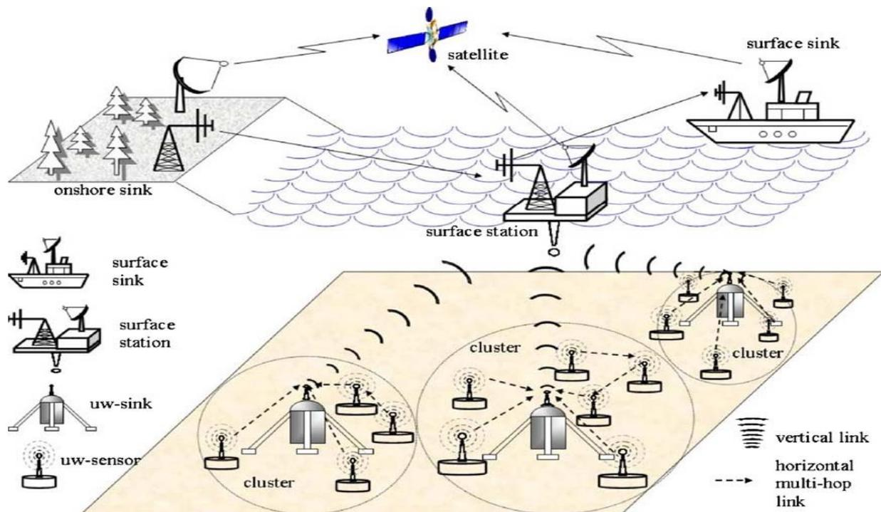
Figure 2.1: 2D Architecture for Underwater Acoustic wireless sensor network adapted from Akyildiz, pompili and medlodia (2005)
