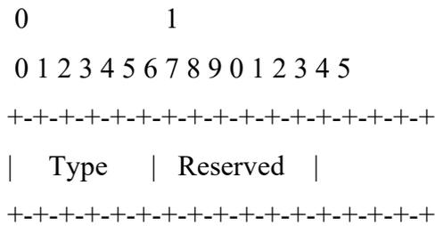
Figure 5.4: RREP -ACK message format for AODV
