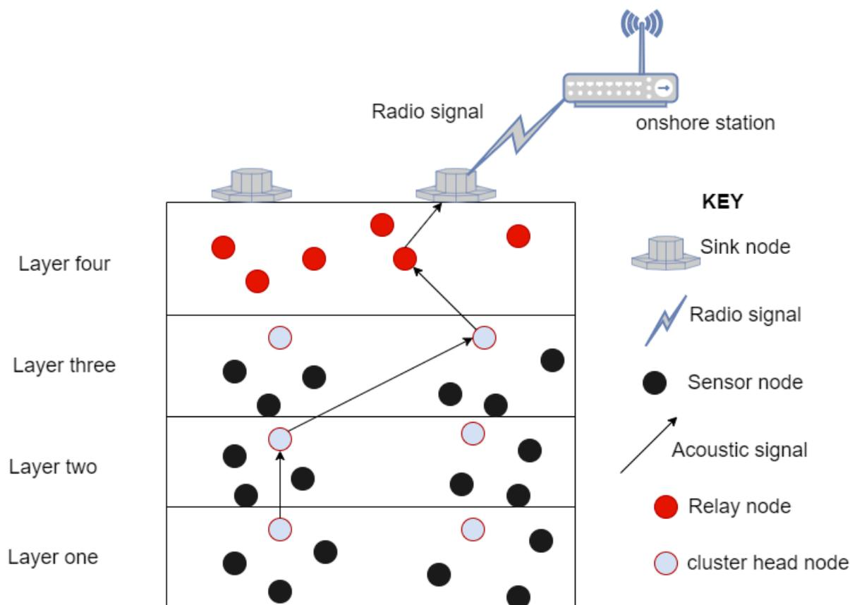
Figure 5.16: Diagram showing the architecture of the proposed dense routing protocol.
