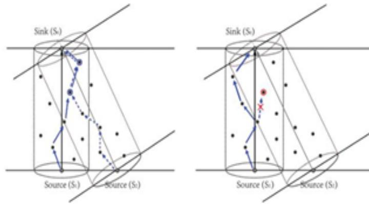
Figure 3.10: Network architecture for VBF and EEC-VBF routing protocols (Tongtong & Ning, 2015)
