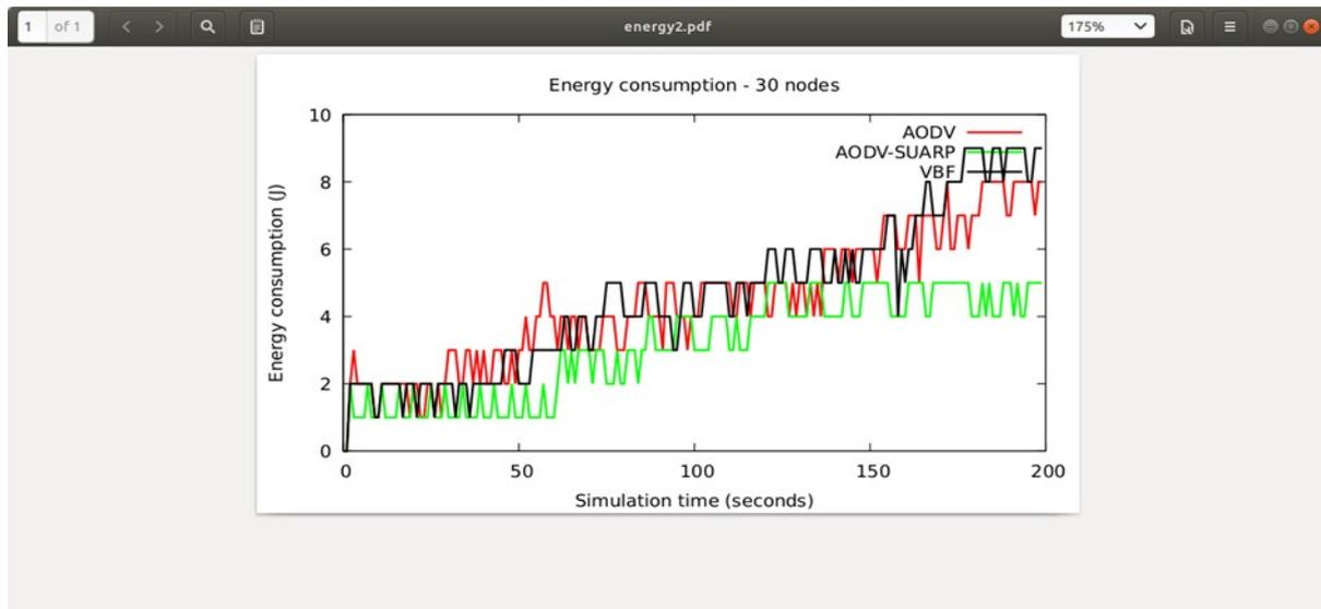
Figure 6.12: Energy consumption for 30 nodes
