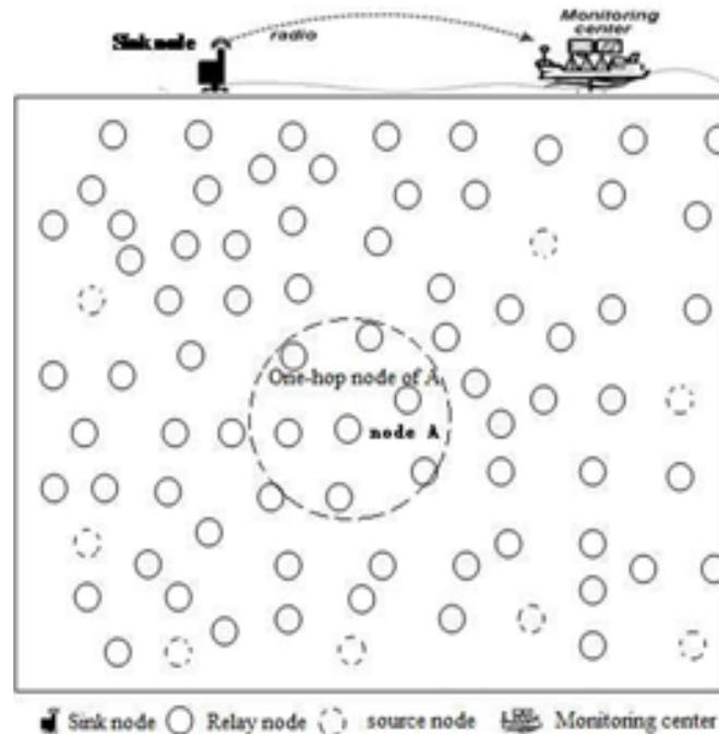
Figure 3.7: Network architecture for the EAVARP routing protocol (Source: Zhuowang et al, 2018)
