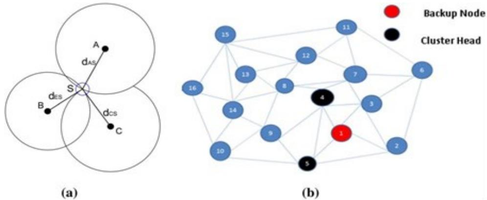
Figure 3.5: (a) The backup node position and (b) The selection of the back-up node (Source: Subrata and Singh 2020)
