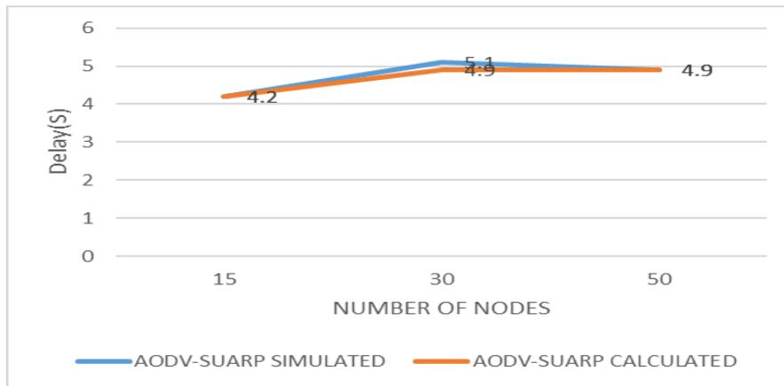
Figure 7.4: Comparison for the simulated and calculated End to End delay for AODV-SUARP
