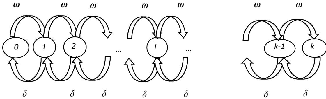
Figure 7.3: Queuing delay for Markov chain based on packet departure (bellalta,2020).
