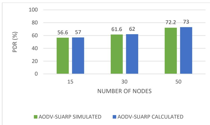
Figure 7.2: Comparison of packet delivery ratio for simulated and calculated AODV-SUARP
