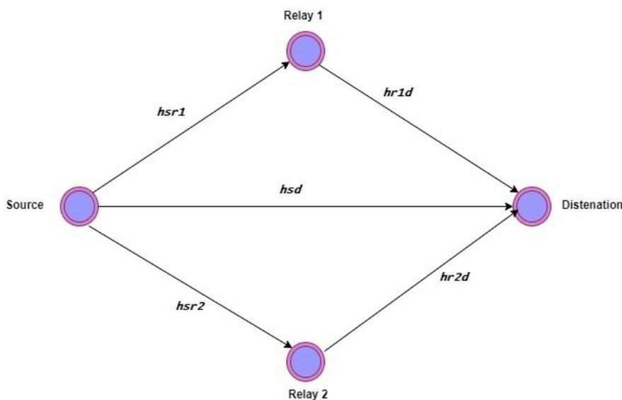
Figure 3.12: Network model of co-operation for CEER routing protocol (Source: Ahmad et al., 2022)
