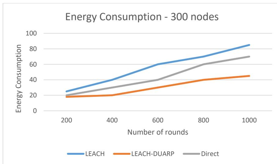
Figure 6.24: Energy consumption for 300 nodes
