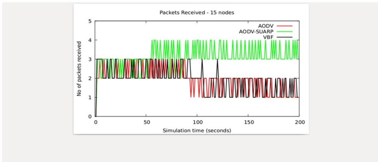
Figure 6.5: Packets received for 15 nodes.
