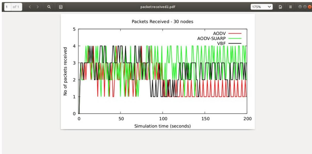
Figure 6.10: Packets received for 30 nodes.
