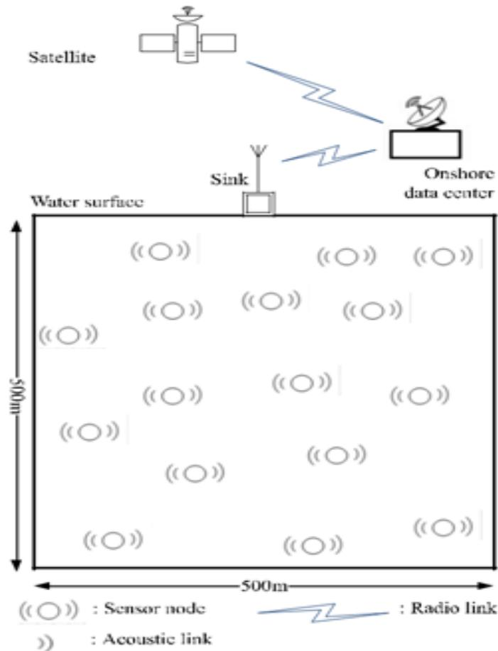
Figure 3.6: Proposed model for CO-EEORS routing protocol (Source: Anwar khan et al (2018))
