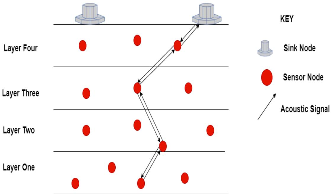
Figure 5.8: Diagram showing the route selection for data forwarding for AODV-SUARP.
