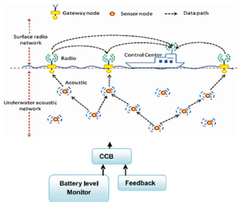
Figure 3.9: Underwater Network Architecture (Source: Ravathi et al, 2019)
