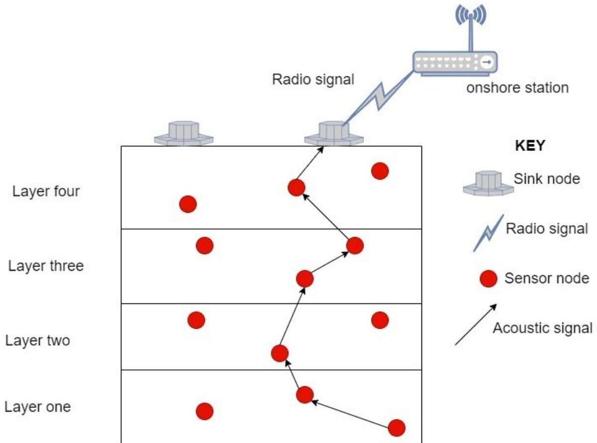
Figure 5.6: Diagram showing the proposed sparse network architecture.
