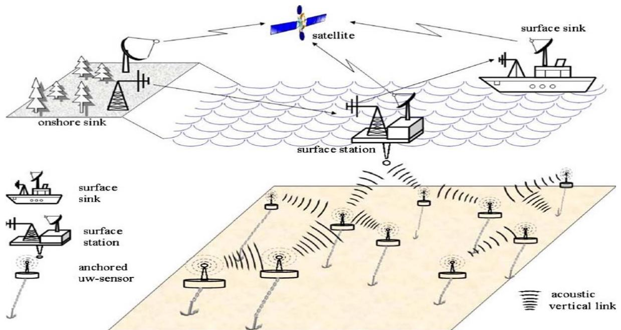
Figure 2.2: 3D Architecture of an underwater acoustic sensor network adapted from Akyildiz, Pompili and Melodia (2005)
